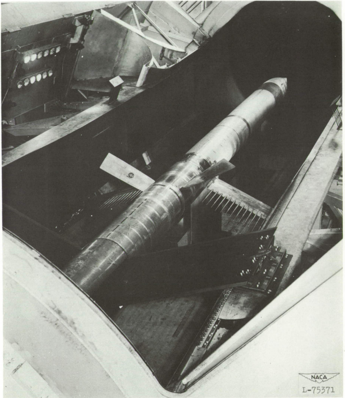
Figure 2.- Propeller mounted on the 6000-horsepower dynamometer in the Langley 16-foot transonic tunnel test section (tunnel open, view looking downstream).
