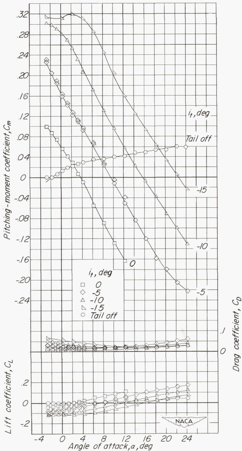
Figure 9.- Wing-off aerodynamic characteristics.
