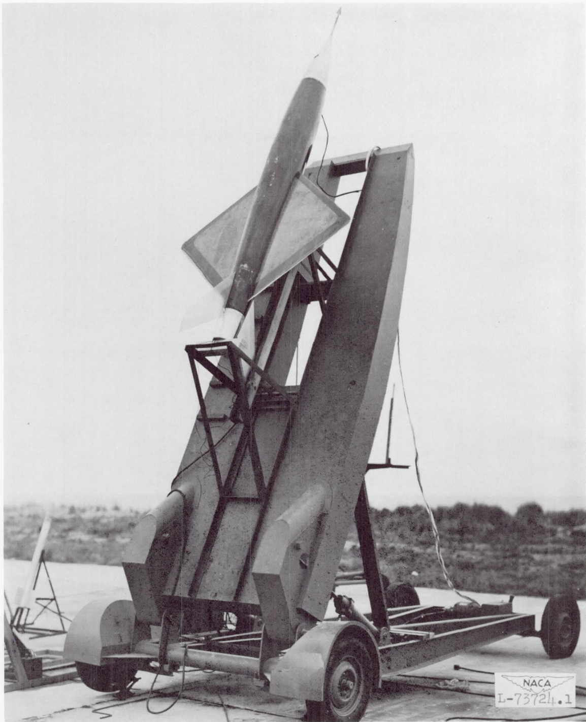
Figure 2.- General view of the model on the launching stand.
