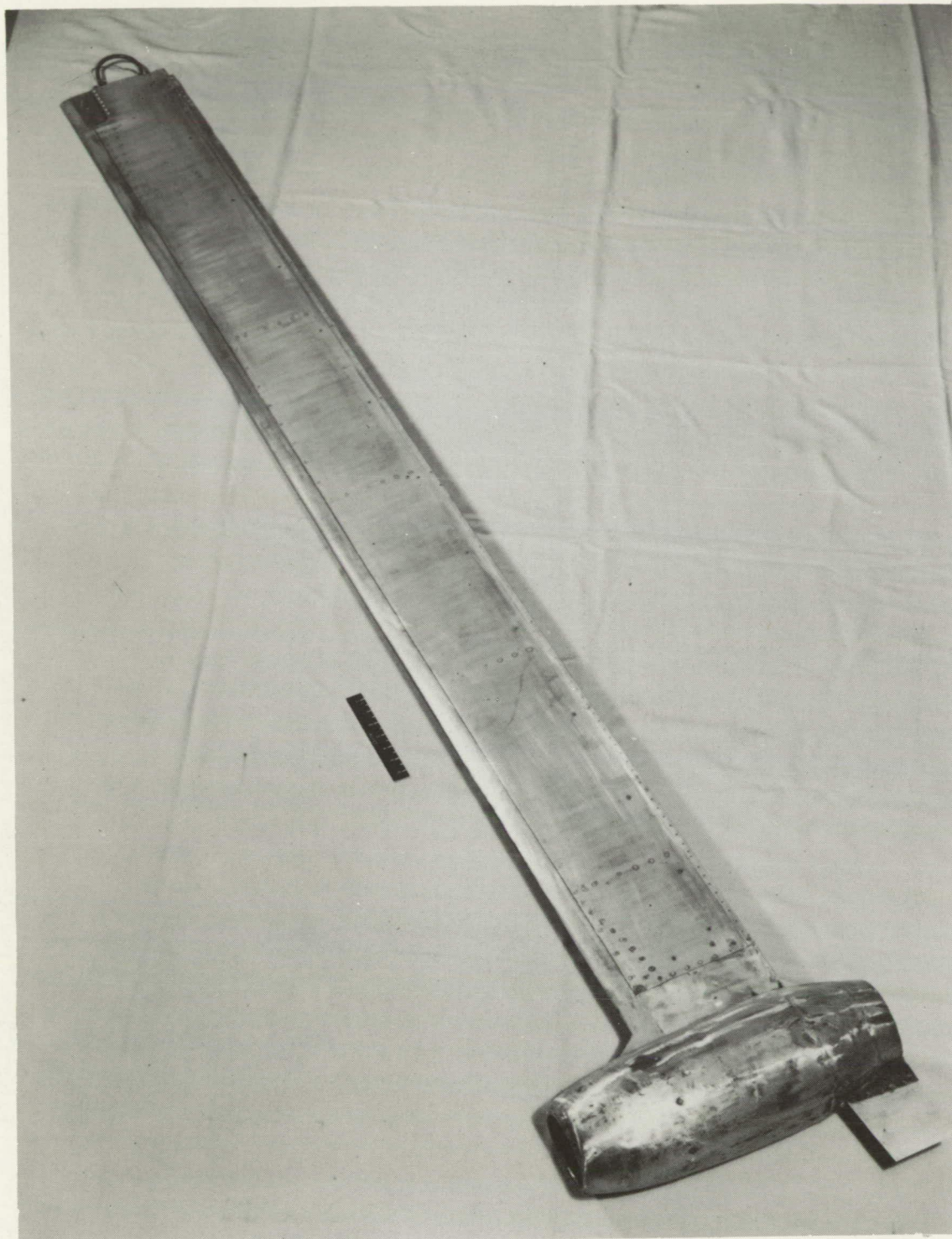
Figure 2.- Outer portion of the engine-blade combination as used for the whirling test on the Langley helicopter test tower.
