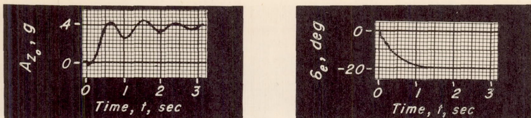
Figure 4.- Optimum response for stabilizing network (no time lag) canceling denominator of airplane transfer function; \dot{\delta}_{eL} = 100^\circ/\text{sec} .
