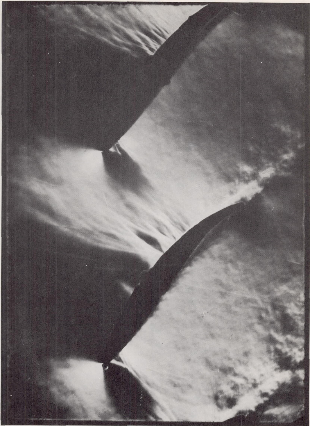
Figure 15.- Schlieren photograph of NACA 65-(12A 2 I 8b )10 blade section at \beta = 60 , \sigma = 1.0 , M = 0.785 , and (\alpha - \alpha_d) = 0.4^\circ .
