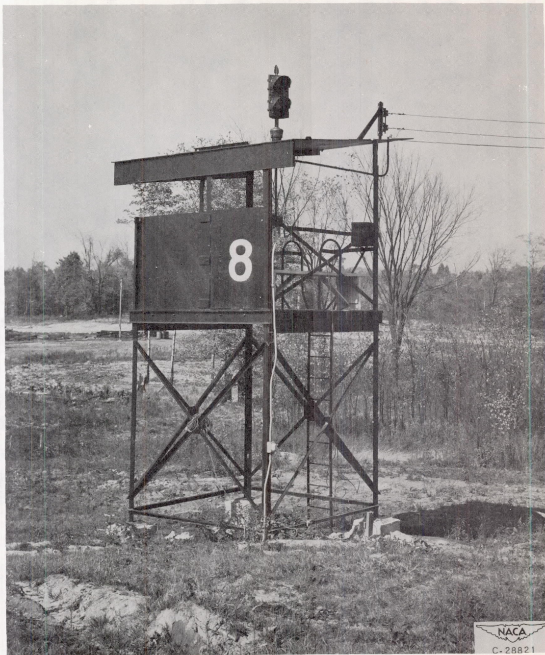
Figure 18. - Typical camera platform installation in crash area.
