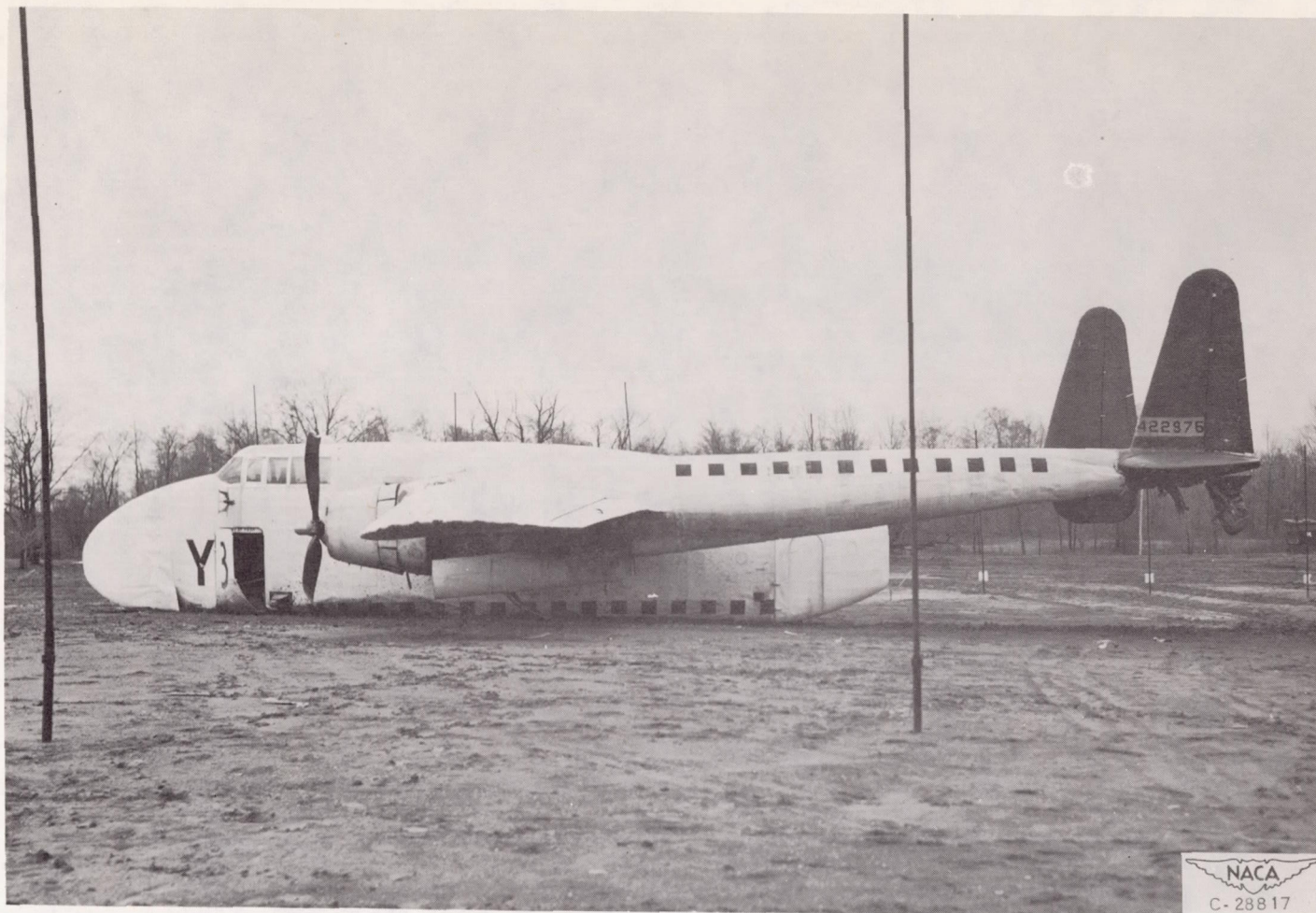
Figure 39. - Black squares painted on side of C-82 airplane and stationary poles in crash area for determining velocity.
