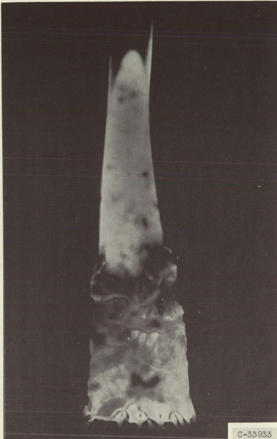
Figure 3. - Propylene diffusion flame burning in 50 percent oxygen, showing formation of solid carbon at base of flame.
