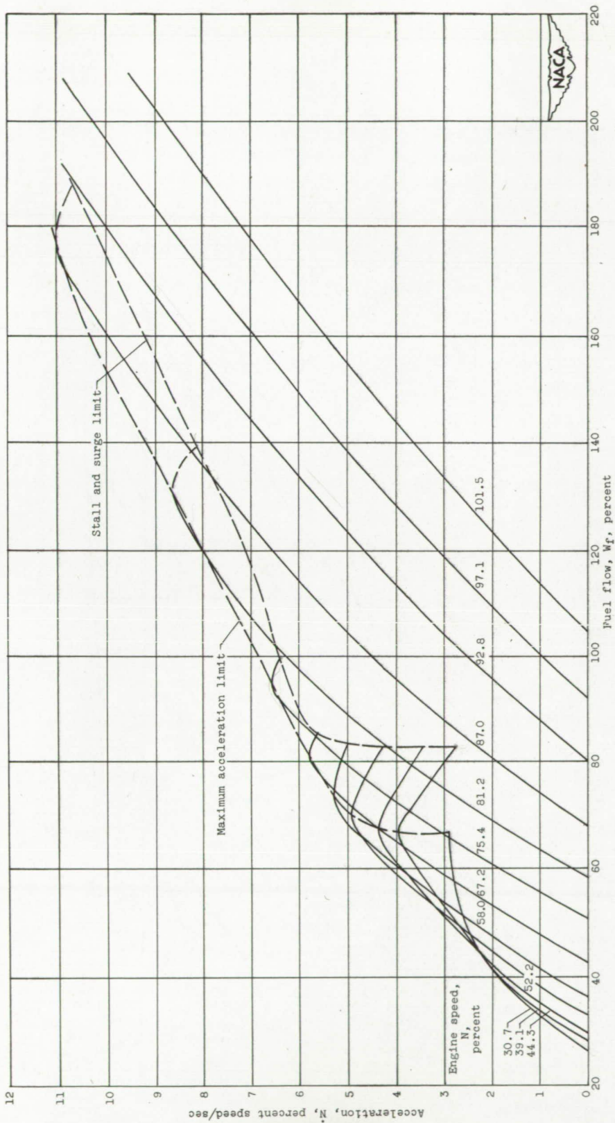
Figure 4. - Acceleration - fuel flow characteristic at constant engine speeds. Parameters shown given in percentage of value at rated rpm at 15,000-foot altitude and 1.02 ram-pressure ratio.
