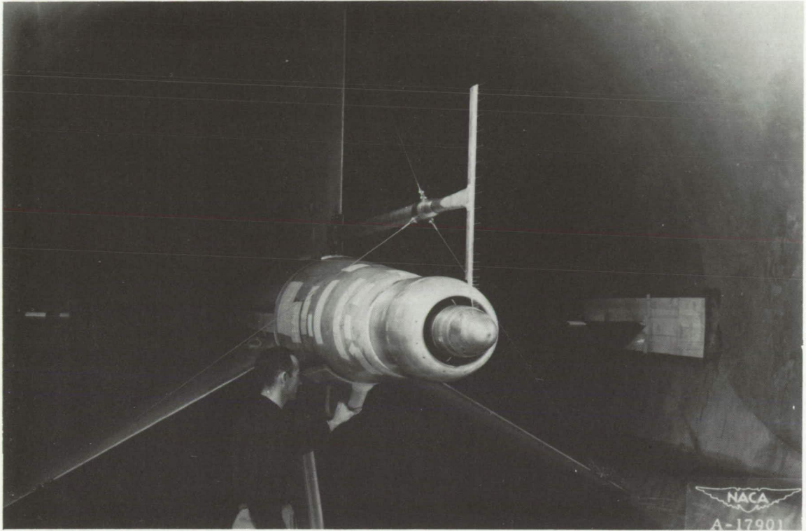
Figure 4.- Photograph of the survey rake.
