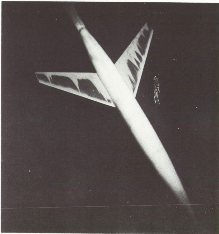
Figure 4.- View of basic model with fluorescent lacquer showing regions of laminar and turbulent boundary-layer flow.
