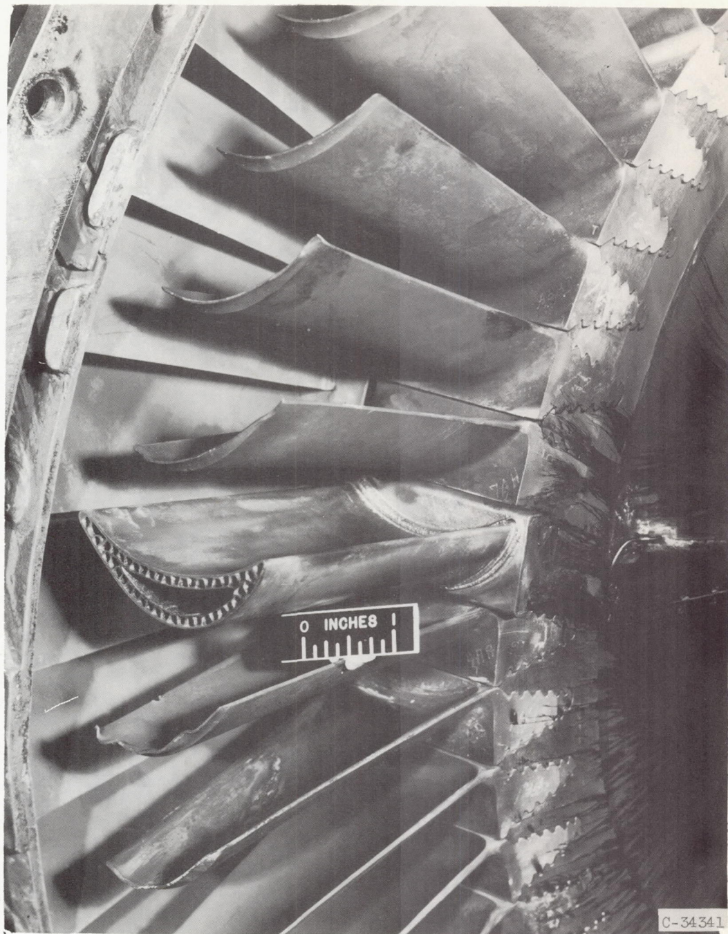
Figure 7. - Sheet-metal bulb-root-type air-cooled base, design 4, in test rotor after 10 hours of endurance operation.
