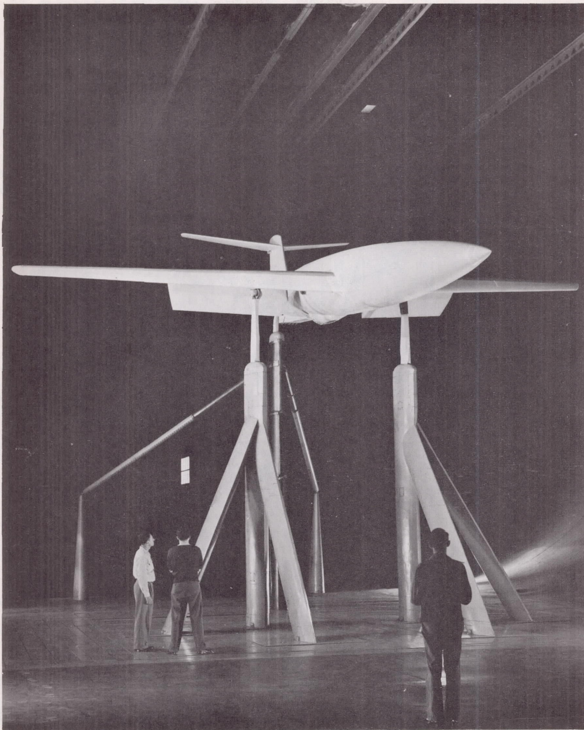
Figure 1.- The 35^\circ sweptback-wing model with the leading-edge and trailing-edge flaps deflected.
