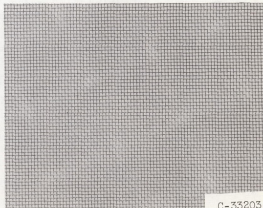
Configuration 5; 28- by 30-inch mesh; 0.013 inch wire diameter.
