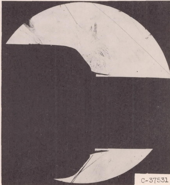
(d) Mass-flow ratio m_3/m_0 , 0.373; total-pressure ratio P_3/P_0 , 0.571.
