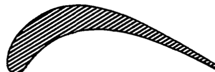
Primary turbine-blade section; \theta_c , 110°; t/c, 15 percent
