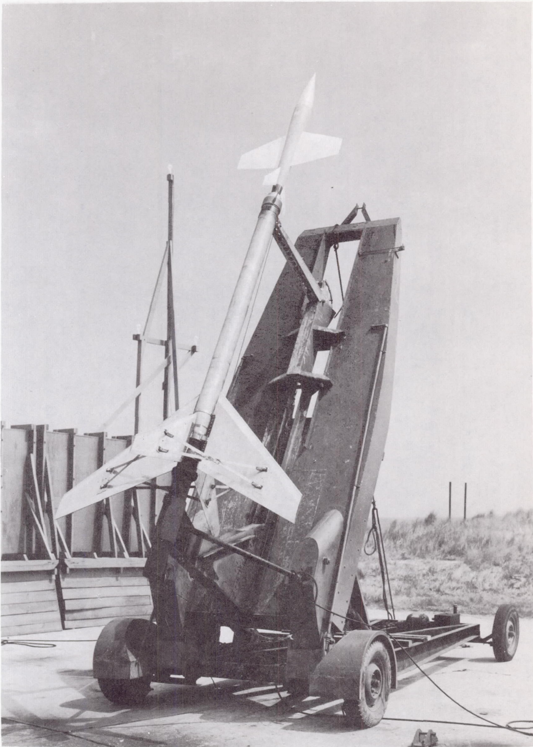
Figure 3.- Photograph of a model and booster on zero-length launcher.
