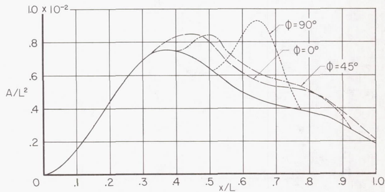
(g) Configuration indented for Mach number 1.41 at M = 1.41 . Model C.
