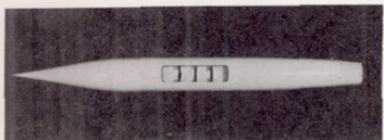
Configuration 3 Box-Type Bomb Bay with Baffles
