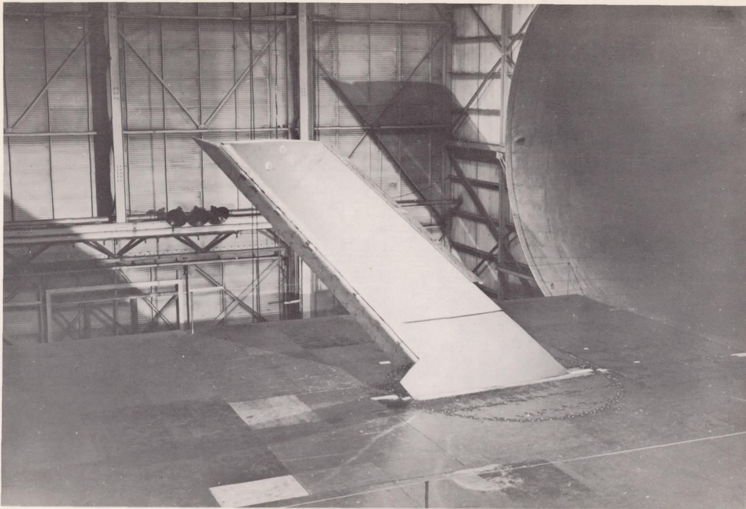
Figure 3.- Photograph of the semispan wing mounted in the Langley full-scale tunnel.
