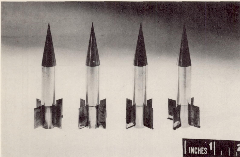
(a) Aileron models with 0, 0.02c, 0.04c, and 0.08c spoiler deflections.
