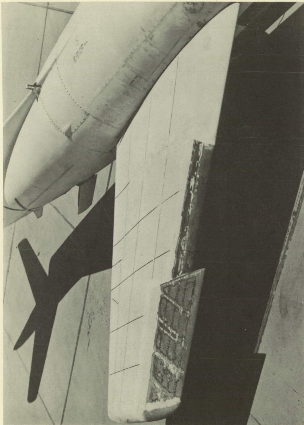
L-87976 Figure 8.- Photograph of the wing of the D-558-II airplane showing the wing leading-edge chord-extension configuration.
