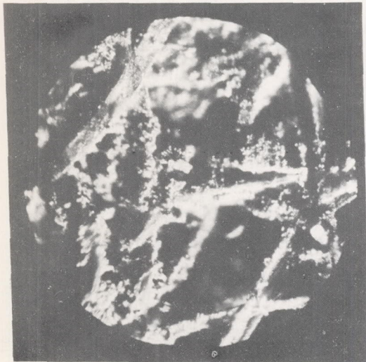
(b) Deposit of fuel D at 400° F; initially saturated with 5 percent oxygen, 95 percent nitrogen mixture.
