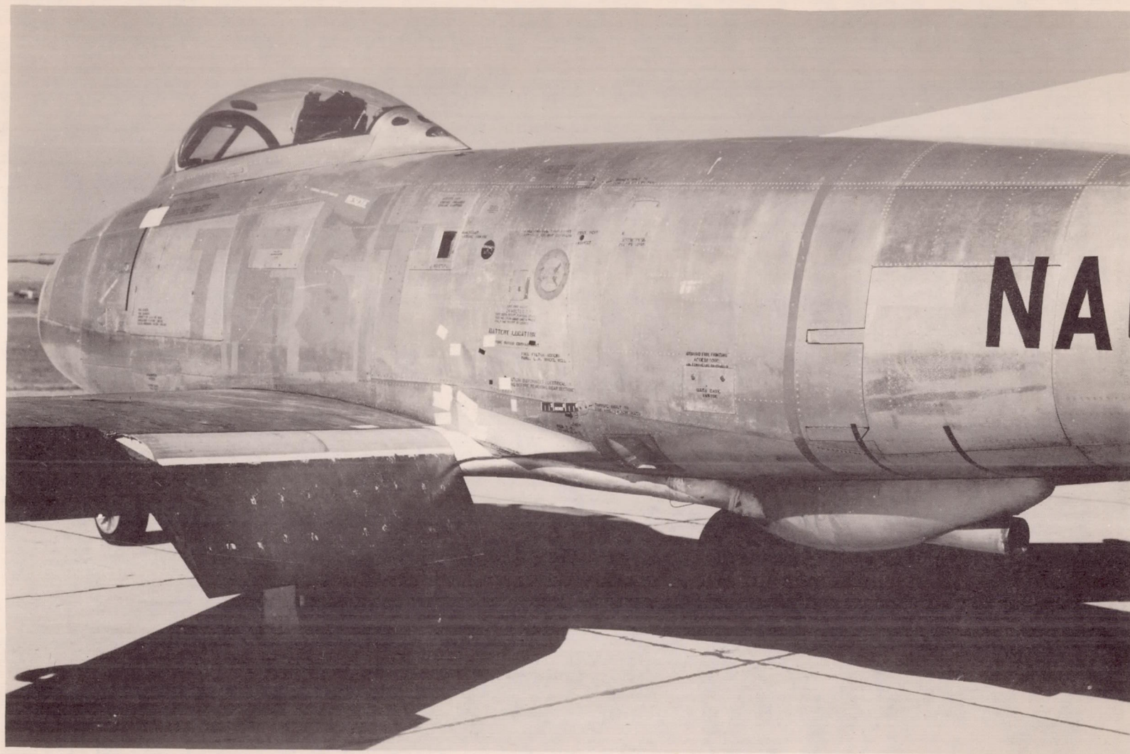
Figure 3.- Close-up showing suction flap, ducts on underside of fuselage, and ejector pump in faired pod.
