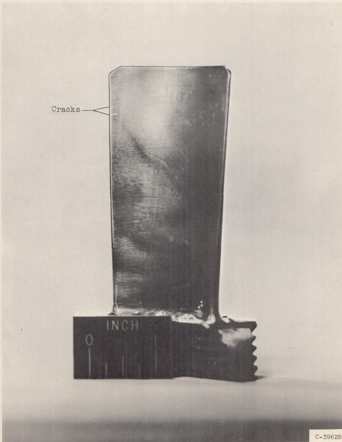
Figure 5. - HS-21 spray-cooled turbine blade with cracks in trailing edge after 10 cycles of operation with gradual water injection.
