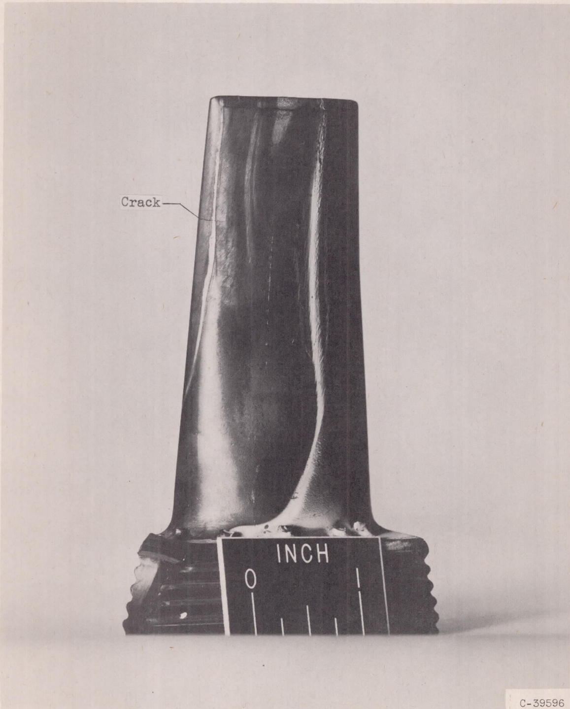
Figure 6. - Inconel X spray-cooled blade with crack in leading edge after 10 cycles of operation with gradual water injection.
