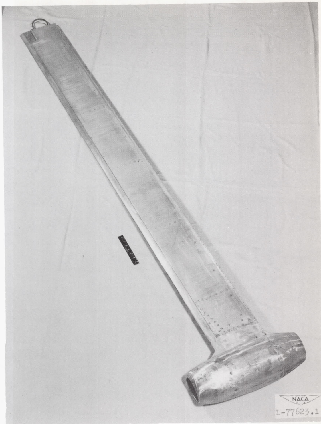
Figure 2.- Ram-jet engine-blade combination used for whirling tests on helicopter test tower.
