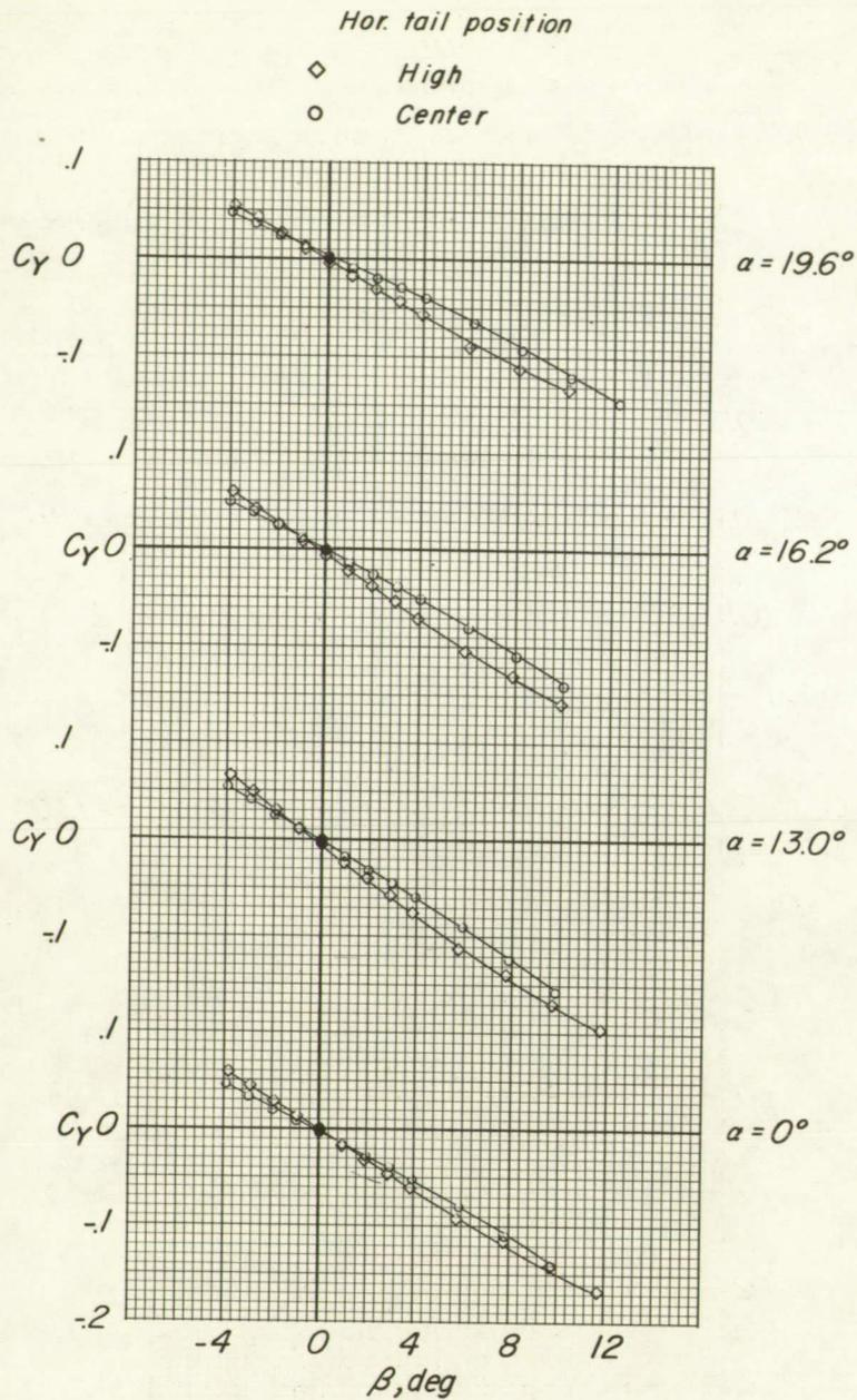
Figure 15.- Variation of lateral aerodynamic characteristics with angle of sideslip at various angles of attack of high-wing-fuselage model with horizontal tail in center and high positions.  $M = 0.85$ .
