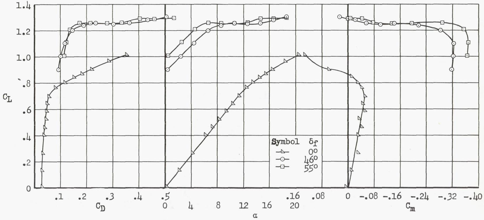
(c) Flap span extending from 0.12 to 0.83 b/2.
