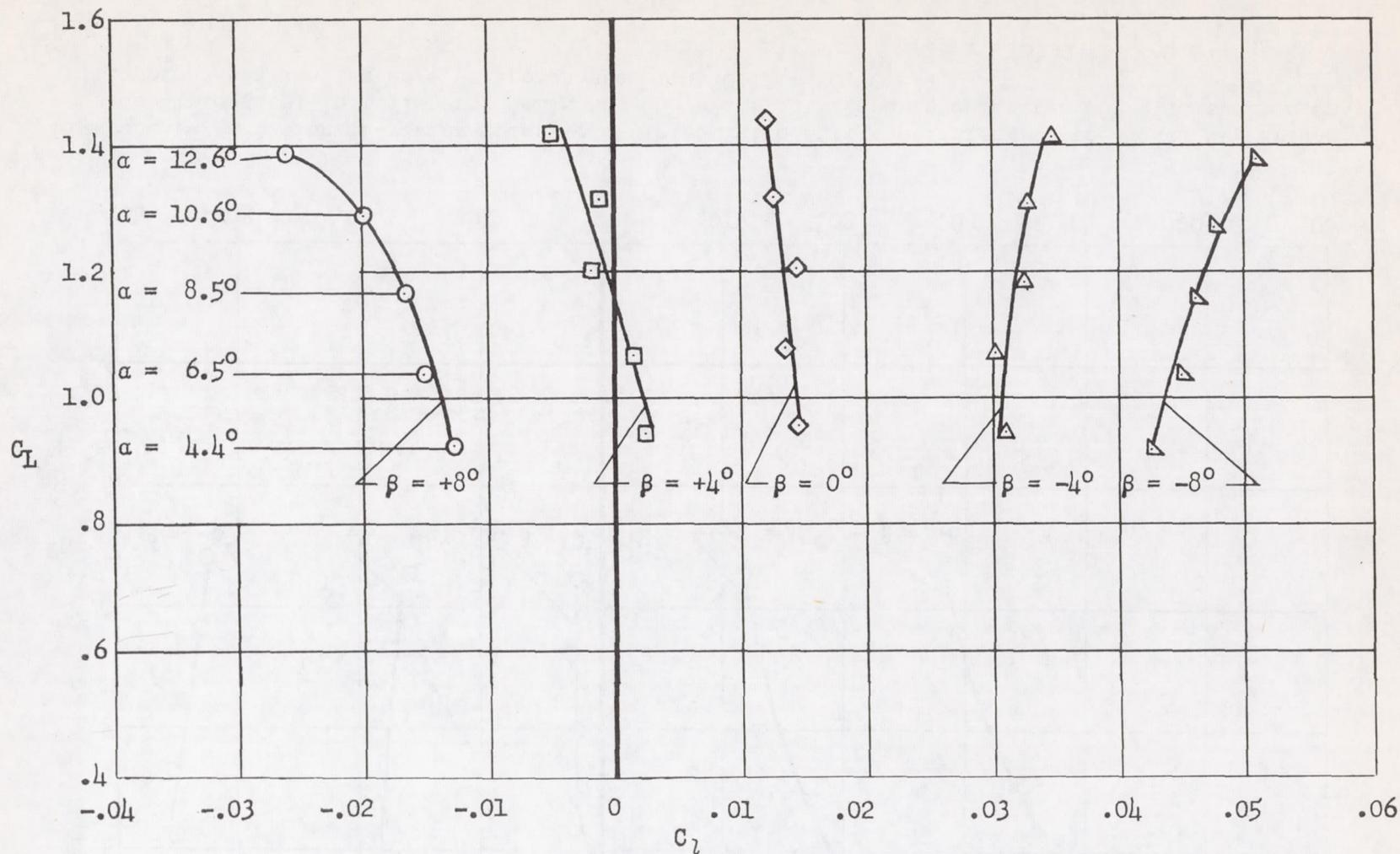
Figure 20.- Variation of rolling-moment coefficient with lift coefficient of the model at various sideslip angles; left flaperon deflected  $65^\circ$  and right flaperon deflected  $46^\circ$ , boundary-layer control applied to the flaperons and leading edge, flaperon span from 0.12 to 0.50  $b/2$ .
