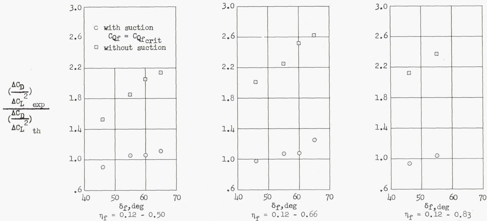
Figure 13.- Effect of suction on the drag parameter  $(\Delta C_D/\Delta C_L^2)_{\text{exp}}/(\Delta C_D/\Delta C_L^2)_{\text{th}}$  for all flap configurations at zero angle of attack.
