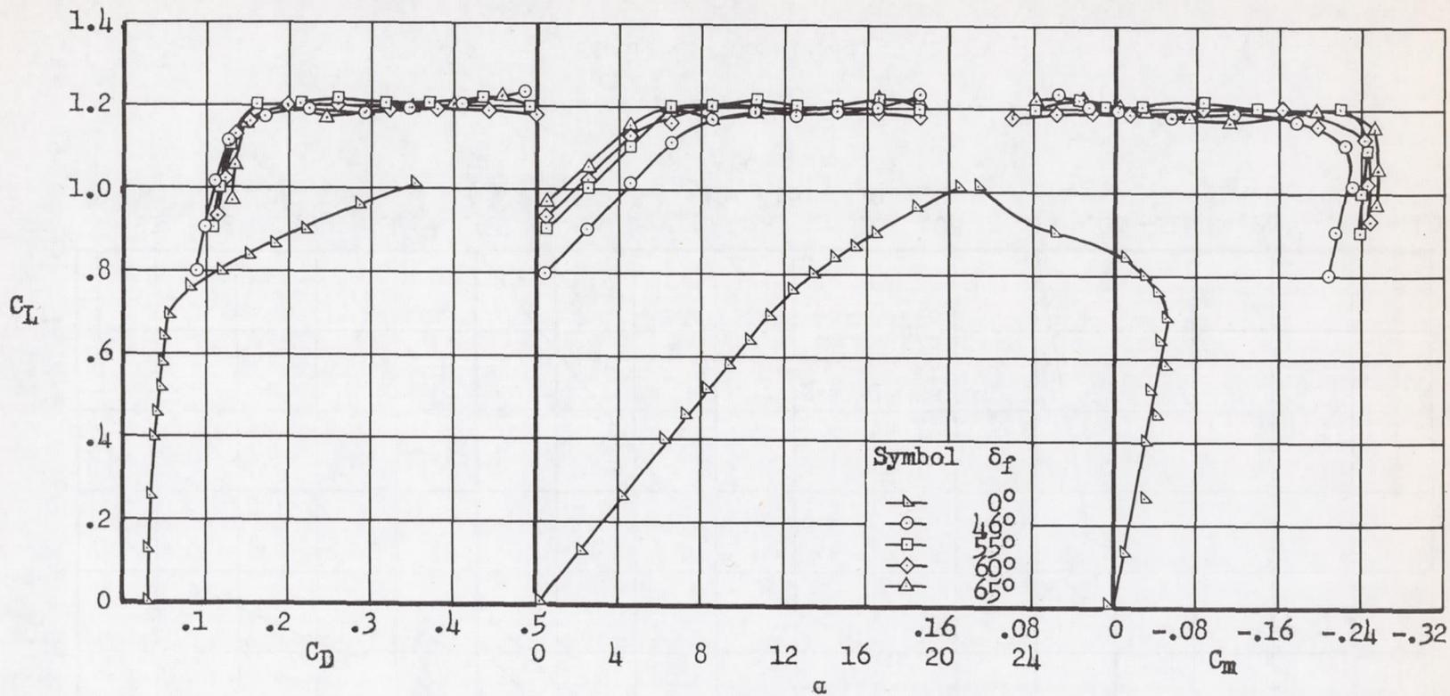
(b) Flap span extending from 0.12 to 0.66  $b/2$ .
