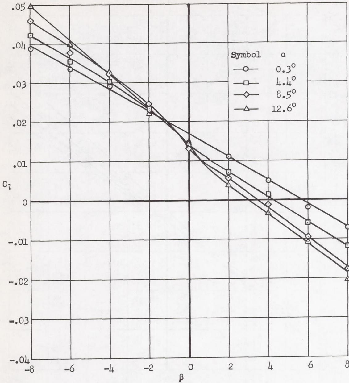
Figure 18.- Variation of rolling-moment coefficient with sideslip angle of the model at various angles of attack; left flaperon deflected  $65^\circ$  and right flaperon deflected  $46^\circ$ ; boundary-layer control applied to flaperons and leading edge; flaperon span from 0.12 to 0.50  $b/2$ .
