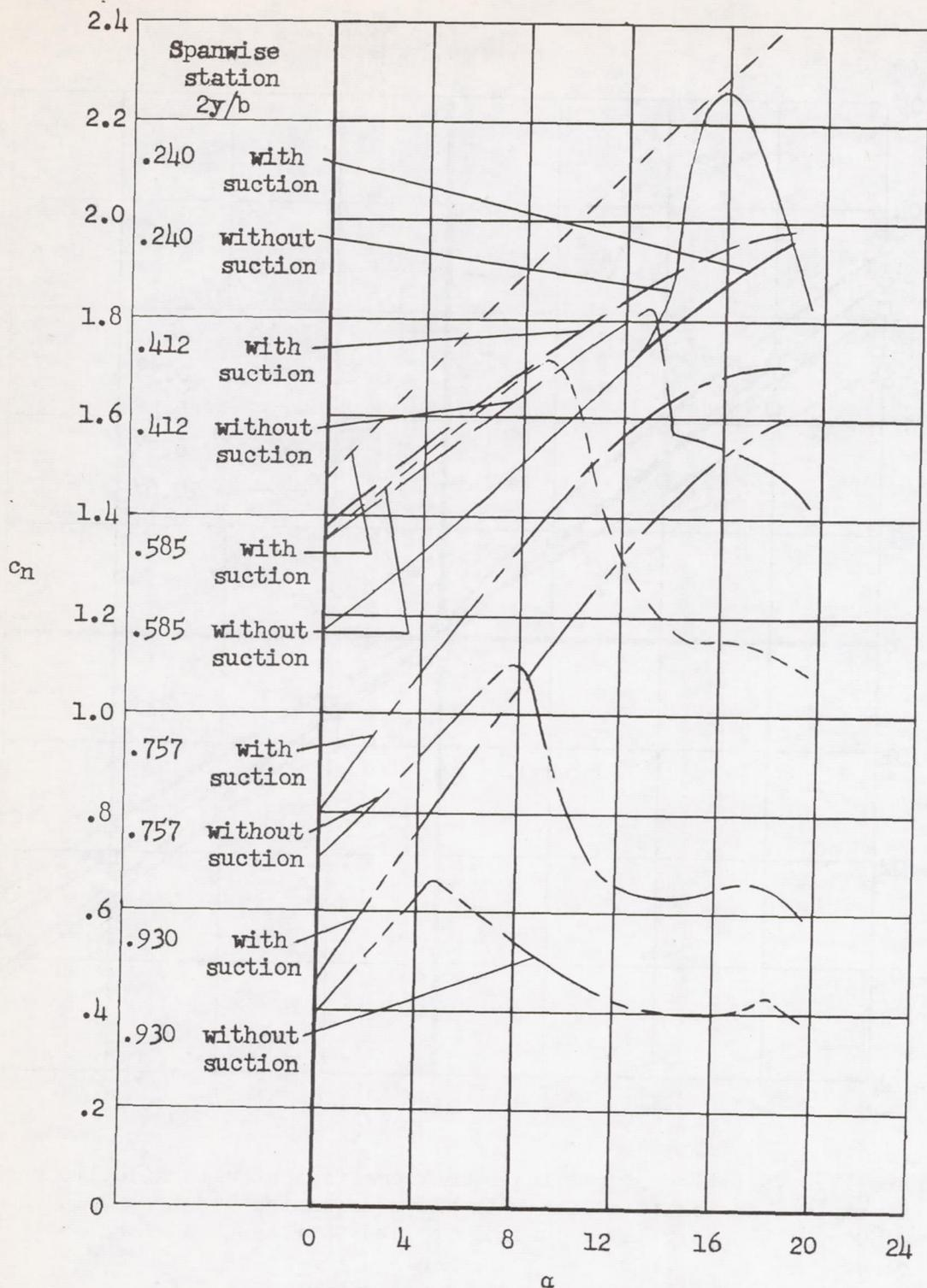
Figure 16.- Effect of area suction at the wing leading edge on the section normal-force coefficient curves for five spanwise stations on the wing with suction on the deflected flap;  $\delta_f = 60^\circ$ , flap span from 0.12 to 0.66  $b/2$ .
