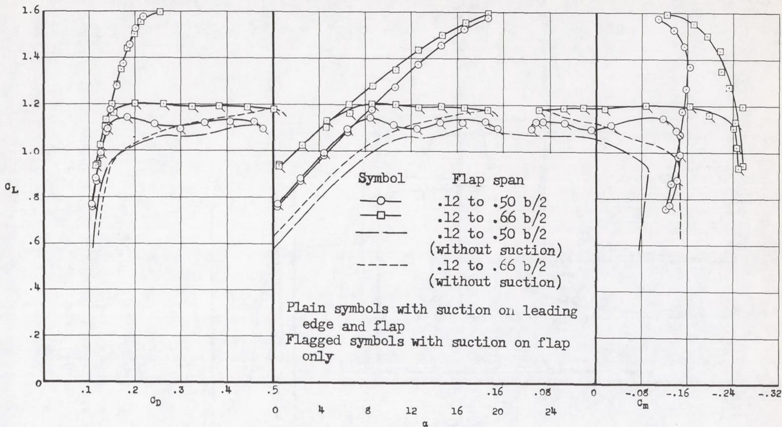
Figure 14.- Effect of leading-edge area suction on the aerodynamic characteristics of the model with area suction applied to each of two flap spans.
