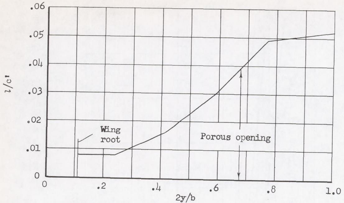
(a) Spanwise variation of chordwise extent of porous area at the wing leading edge.
