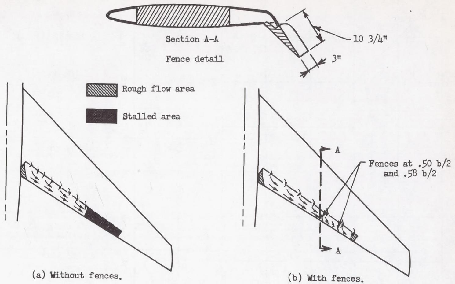
Figure 9.- Tuft study of the flow over the flaps with suction on the flap;  $\delta_f = 65^\circ$ , flap span from 0.12 to 0.66  $b/2$ .
