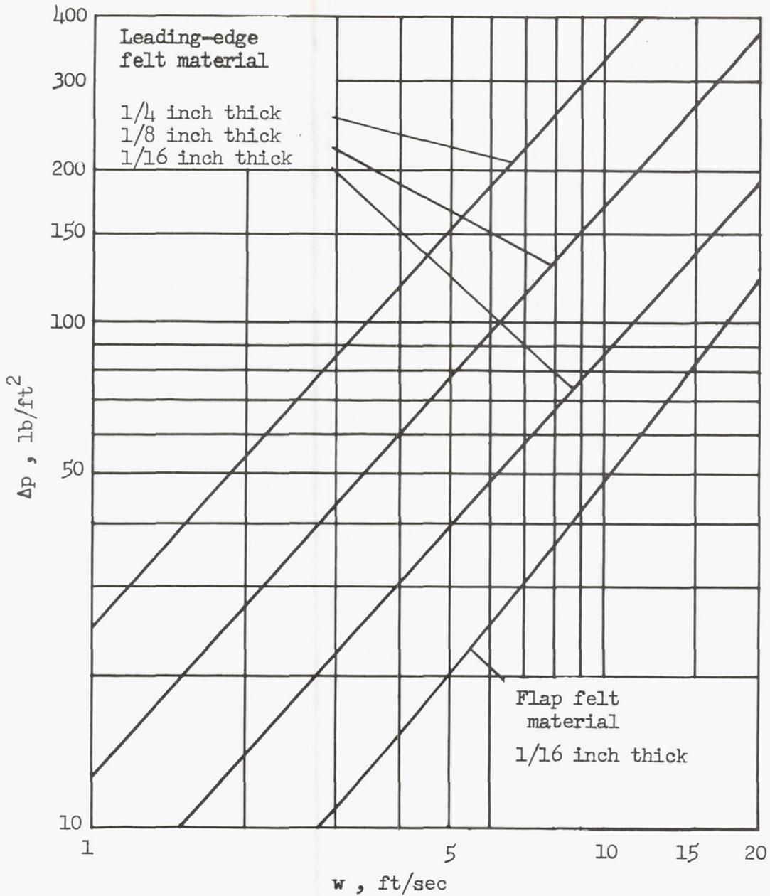
Figure 4.- Porosity characteristics of the wool felt material used for boundary-layer control.
