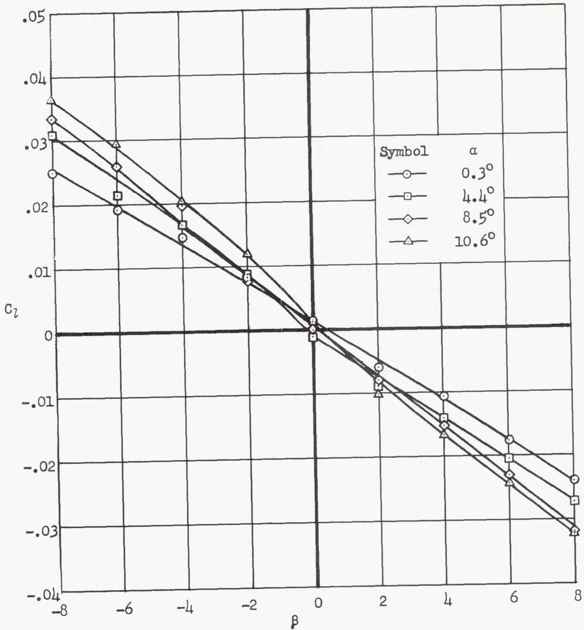
Figure 17.- Variation of rolling-moment coefficient with sideslip angle at various angles of attack with flaps deflected  $55^\circ$  from 0.12 to 0.50  $b/2$ ; boundary-layer control applied to flaps and wing leading edge.
