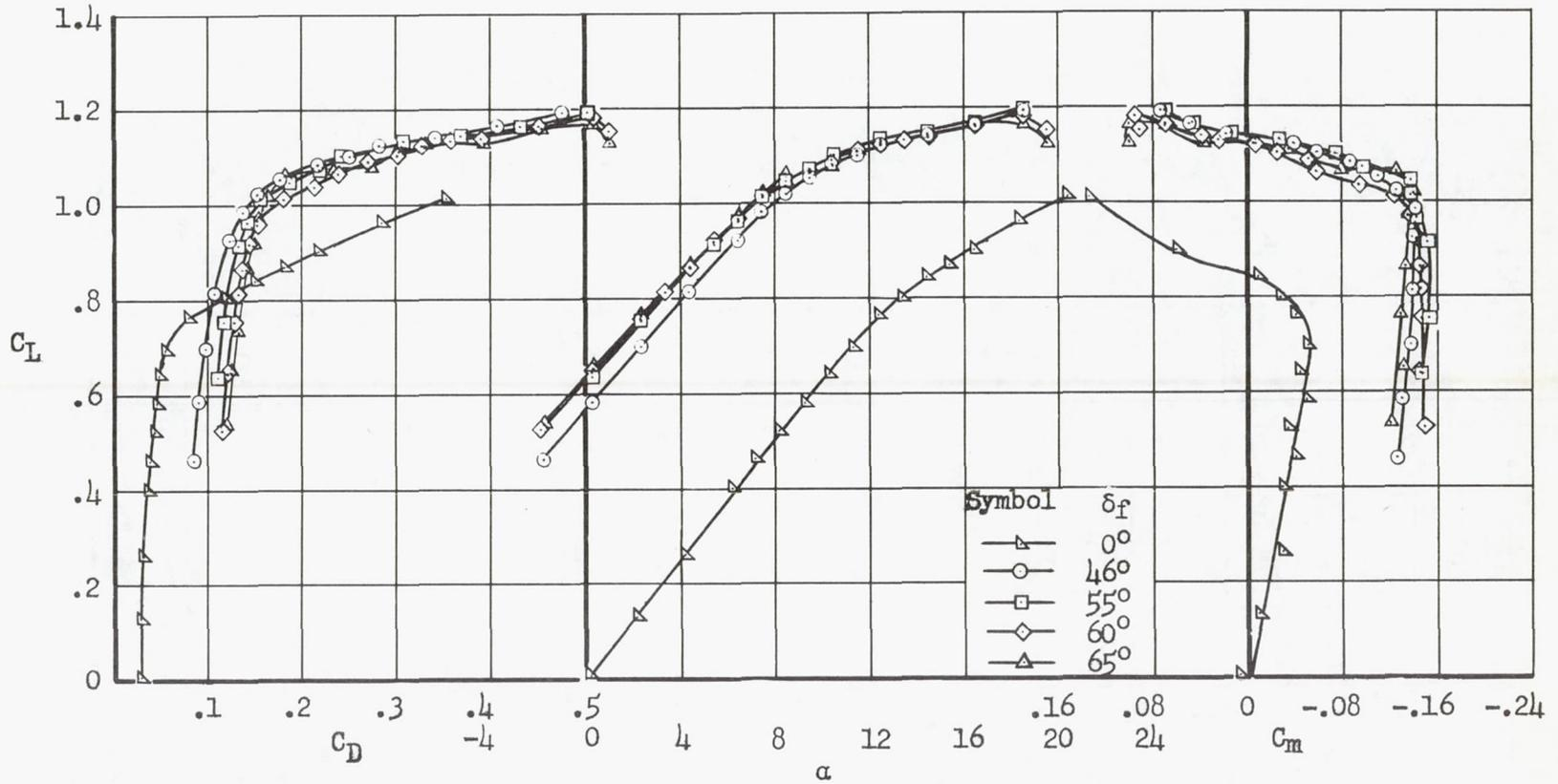
(b) Flap span extending from 0.12 to 0.66  $b/2$ .
