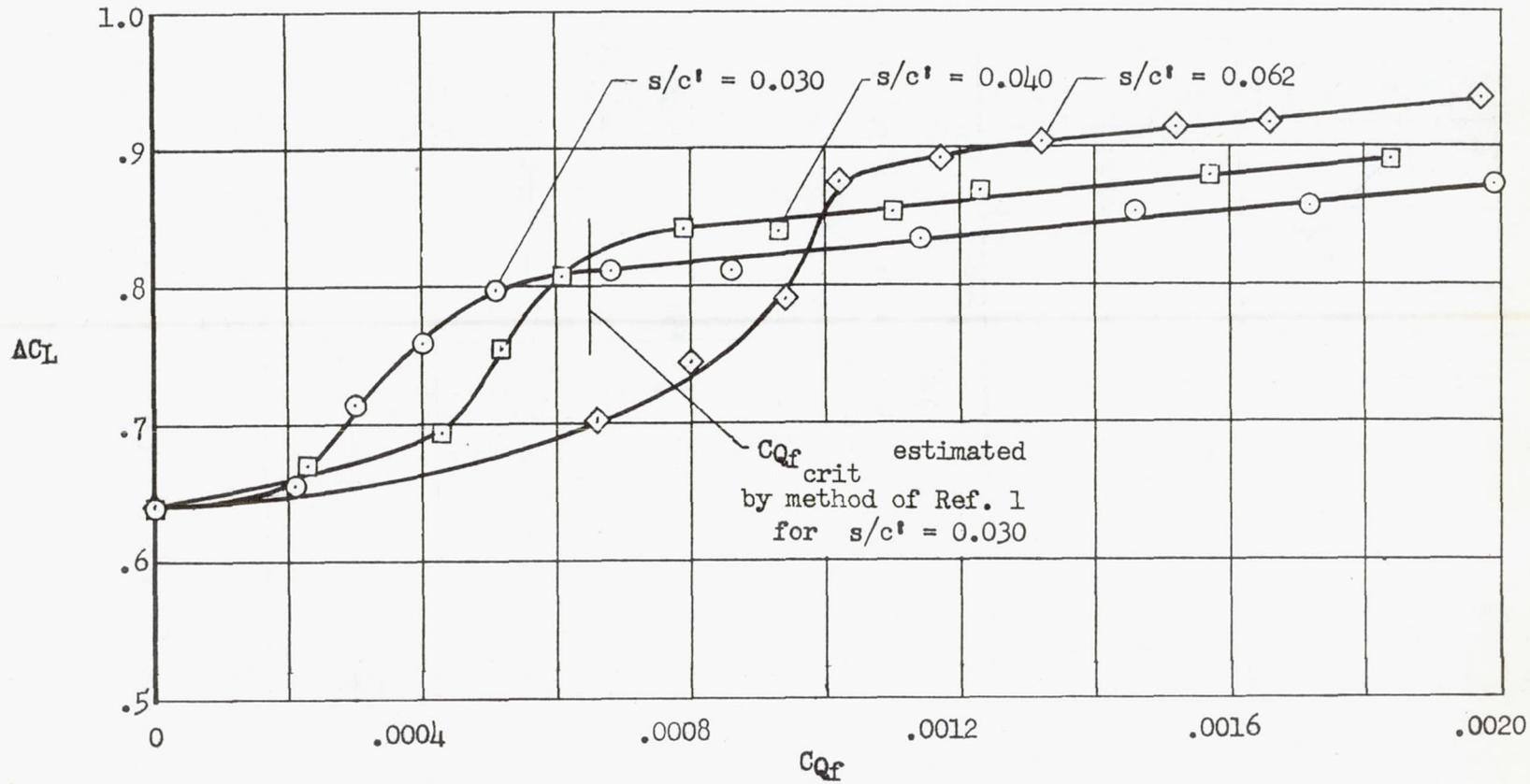
Figure 6.- Effect of flow coefficient on the flap lift coefficient increment for various chordwise extents of porous area;  $\alpha = 0.4^\circ$ ,  $\delta_f = 55^\circ$ , flap span from 0.12 to 0.66  $b/2$ , wing leading edge sealed.
