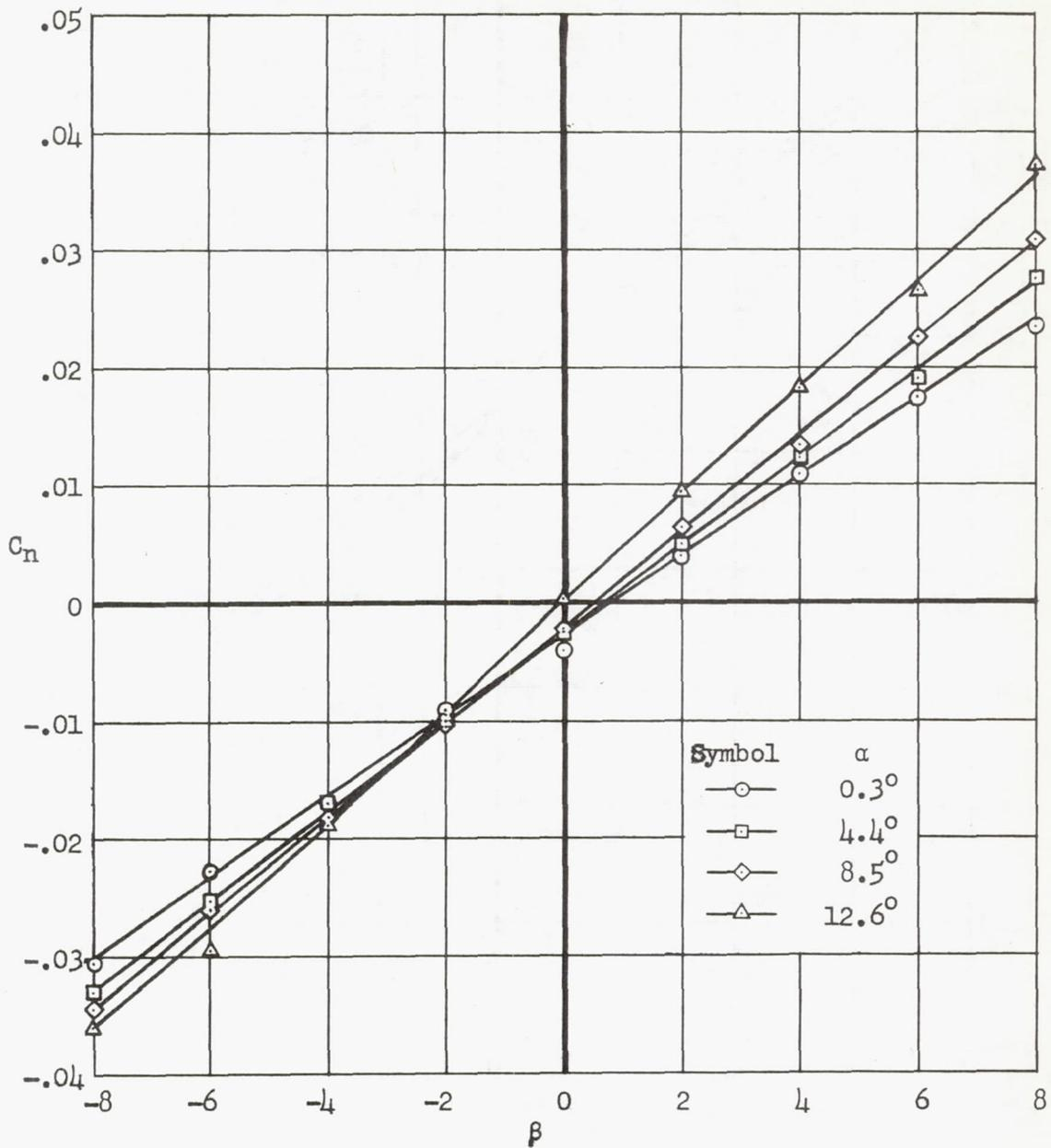
Figure 19.- Yawing-moment coefficient variation with sideslip angle of the model at various angles of attack; left flaperon deflected  $65^\circ$  and right flaperon deflected  $46^\circ$ ; boundary-layer control applied to flaperons and leading edge; flaperon span from 0.12 to 0.50  $b/2$ .
