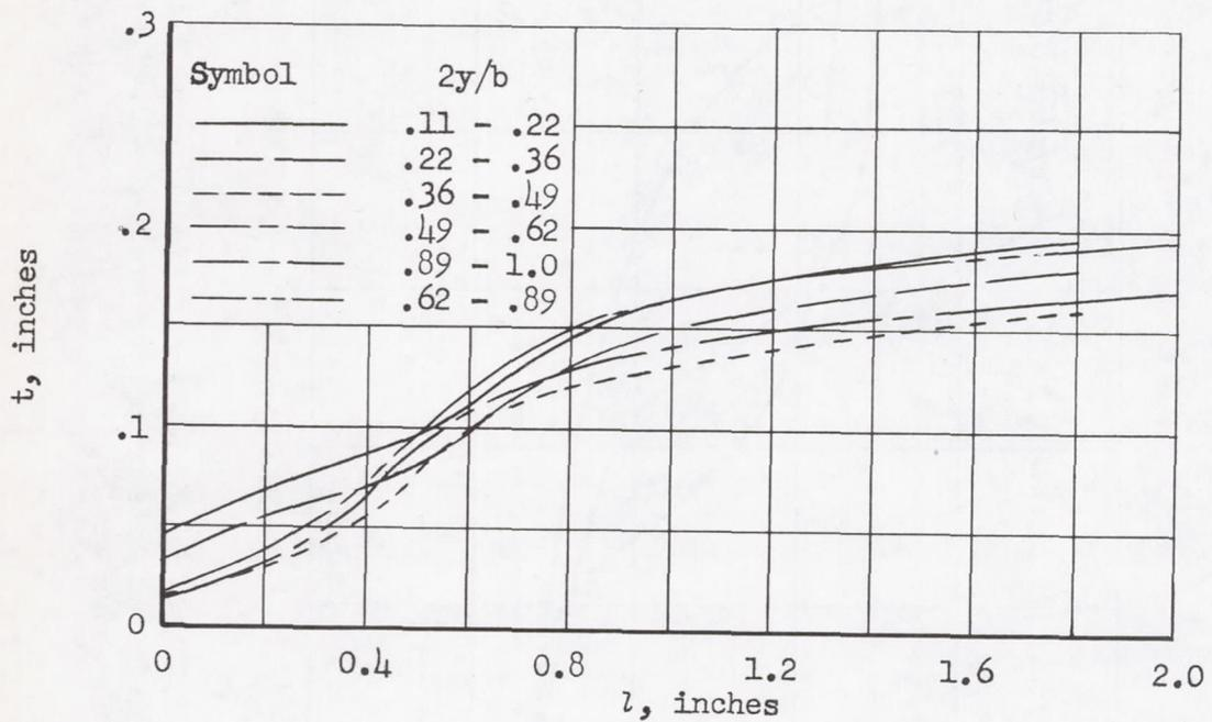
(b) Thickness variation of the felt backing used in the wing leading edge.
