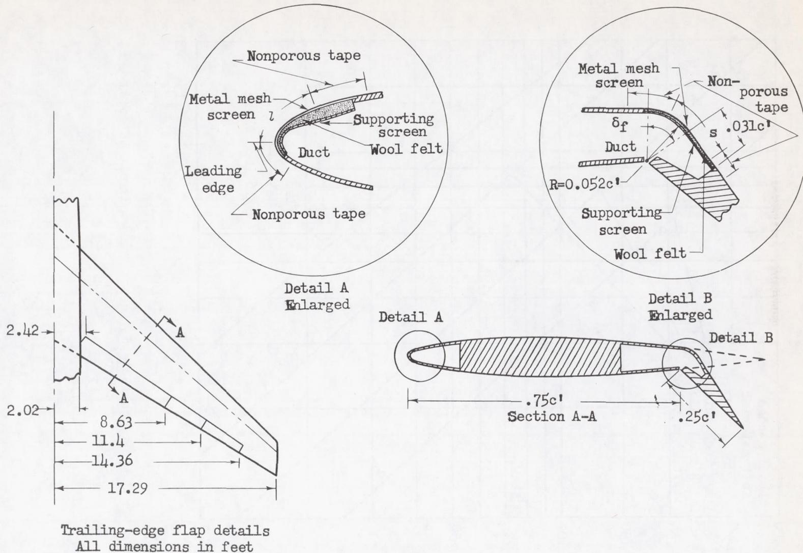
Figure 3.- Details of the flap and leading edge of the model.
