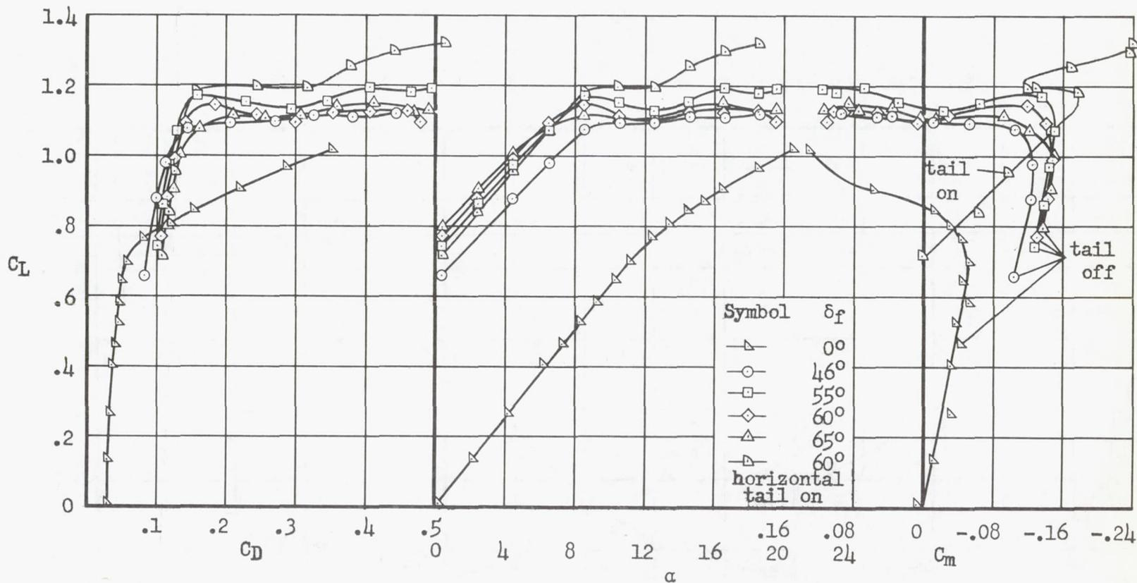
(a) Flap span extending from 0.12 to 0.50  $b/2$ .
