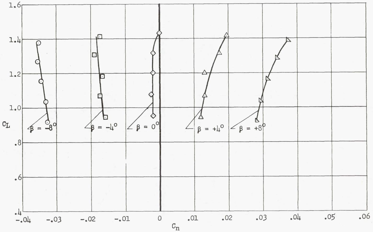
Figure 21.- Variation of yawing-moment coefficient with lift coefficient of the model at various sideslip angles; left flaperon deflected  $65^\circ$  and right flaperon deflected  $46^\circ$  with suction on flaperons and leading edge, flaperon span from 0.12 to 0.50  $b/2$ .
