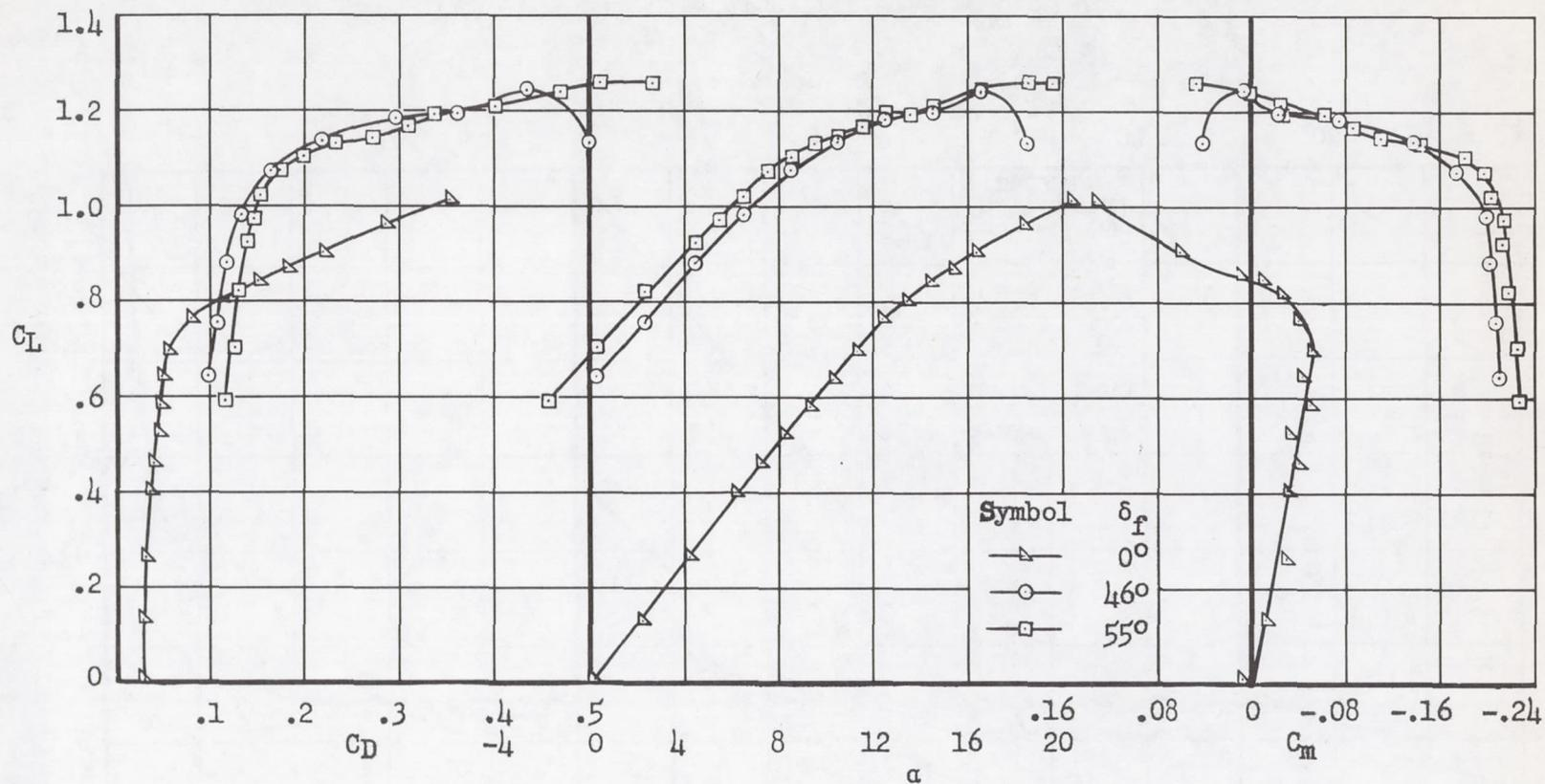
(c) Flap span extending from 0.12 to 0.83  $b/2$ .
