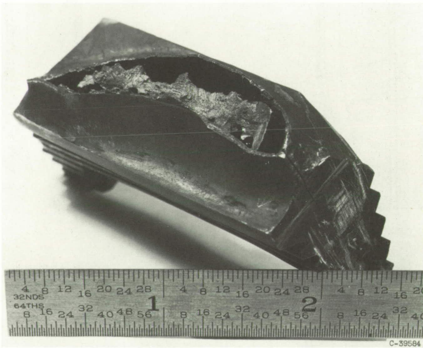
(b) Blade 20, failure after 24 hours.
