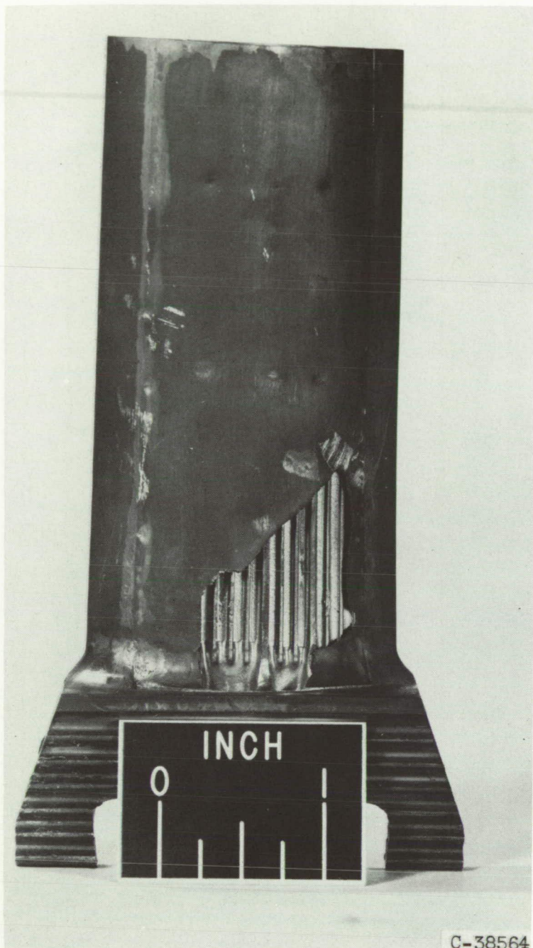
Figure 14. - Shell failure of blade 24 (modification 6) after 18 hours of operation.
