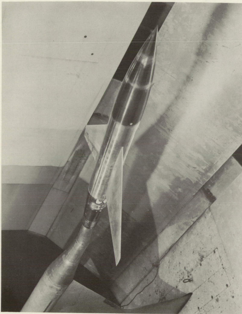
Figure 2.- Model installed in the test section of the Langley 16-foot transonic tunnel. L-87668
