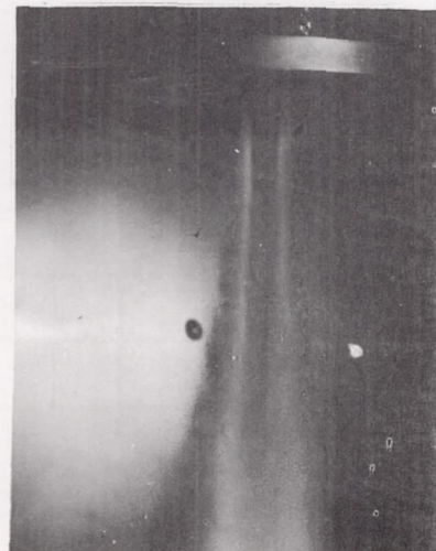
Center jet pressure drop, 250 pounds per square inch.
