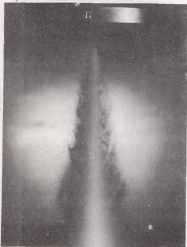
Center jet pressure drop, 250 pounds per square inch.
