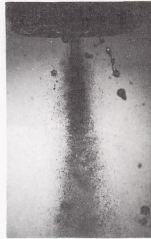
Center sheet pressure drop, 10 pounds per square inch.
