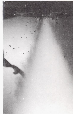
Center sheet pressure drop, 250 pounds per square inch.
