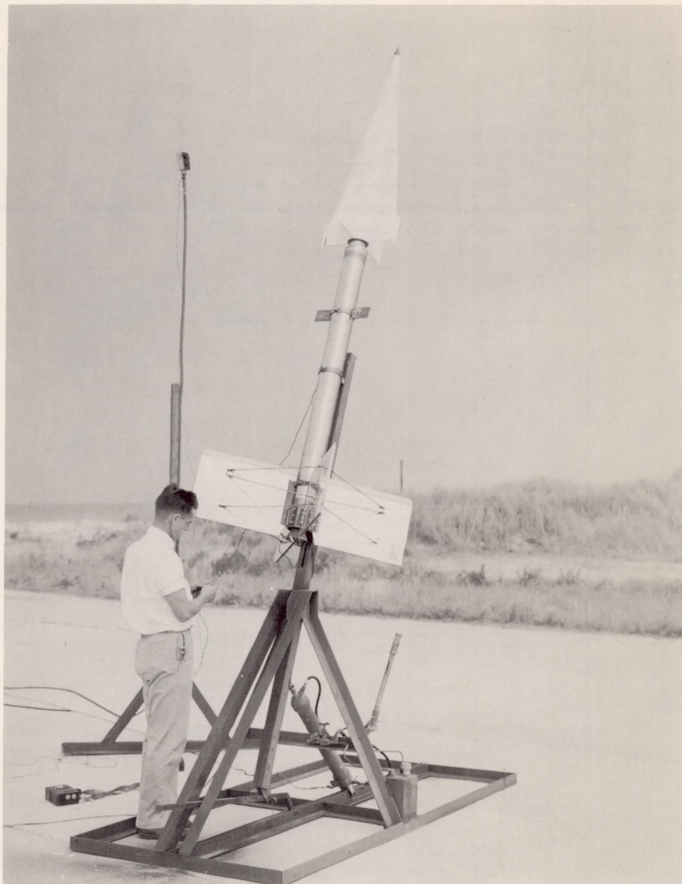
(b) Model 15 mounted with booster on launching stand and being prepared for flight test.
