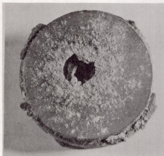
(c) Model 25 (15 minute coating) after 632 seconds testing time. Destruction began at some time after 541 seconds.
