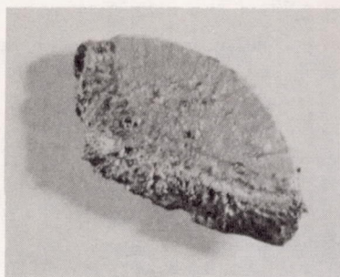
(b) Model 27 (10 minute coating) after 285 seconds testing time. Destruction began at 277 seconds.
