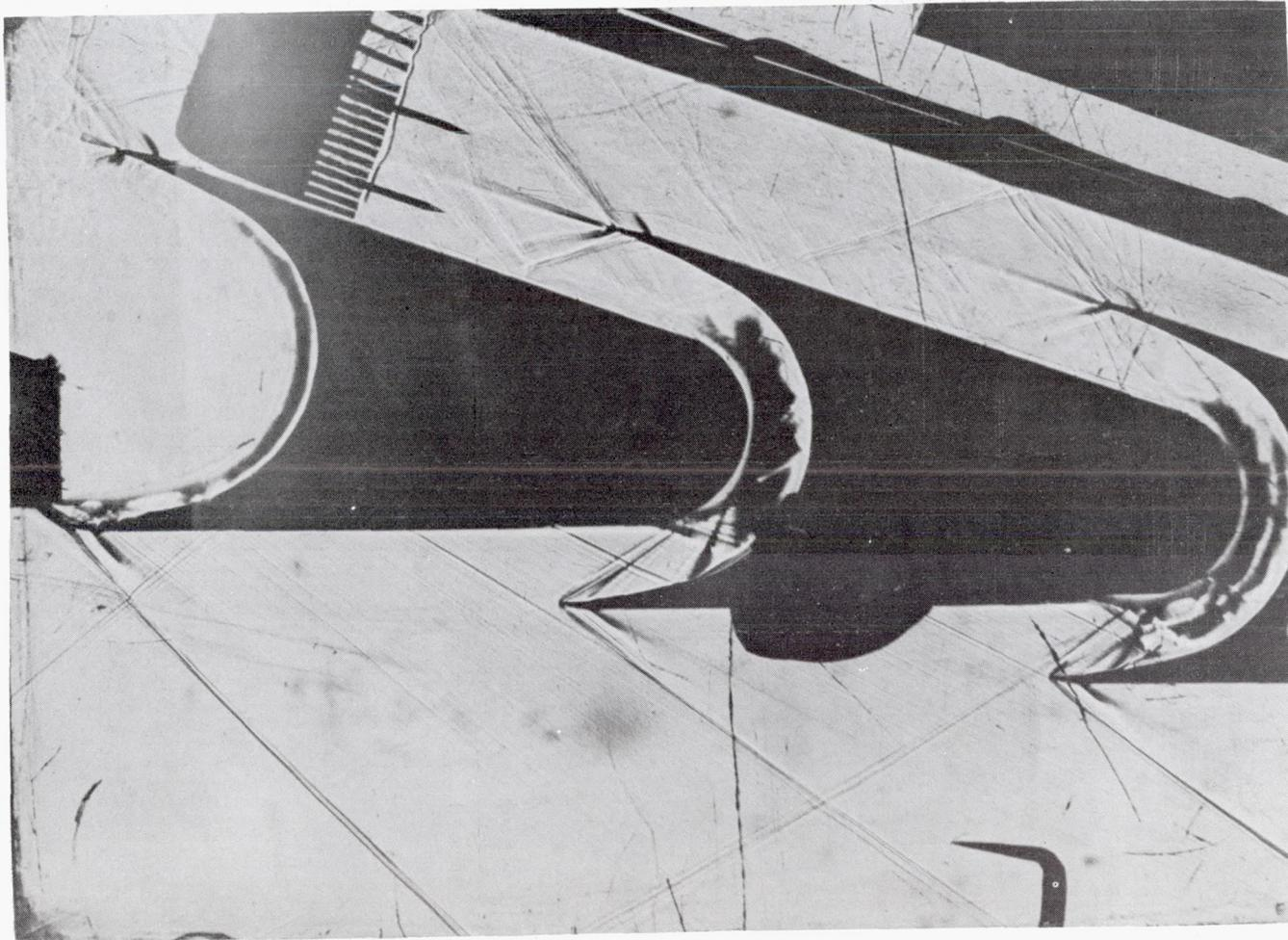
Figure 4.- Schlieren photograph of full-contour blades at a floor angle of  $8.4^\circ$ . Rake is 1.500 inches from tunnel wall.
