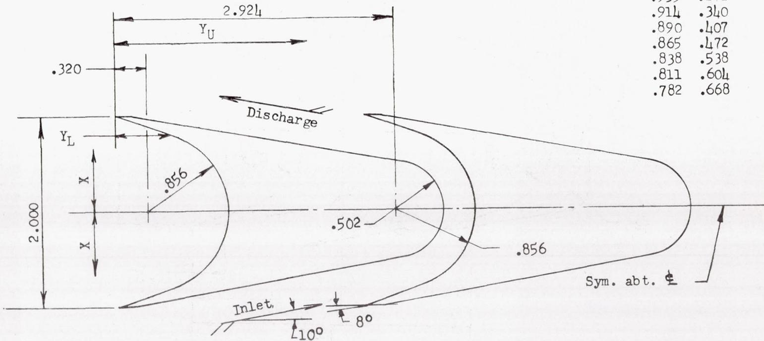
Figure 1.- Full-contour blade sections. All dimensions are in inches unless otherwise indicated.
