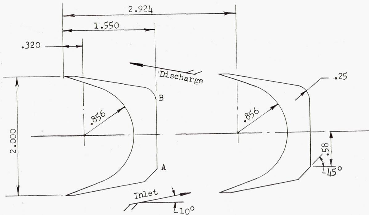
Figure 2.- Free-streamline blade sections. All dimensions are in inches unless otherwise indicated.
