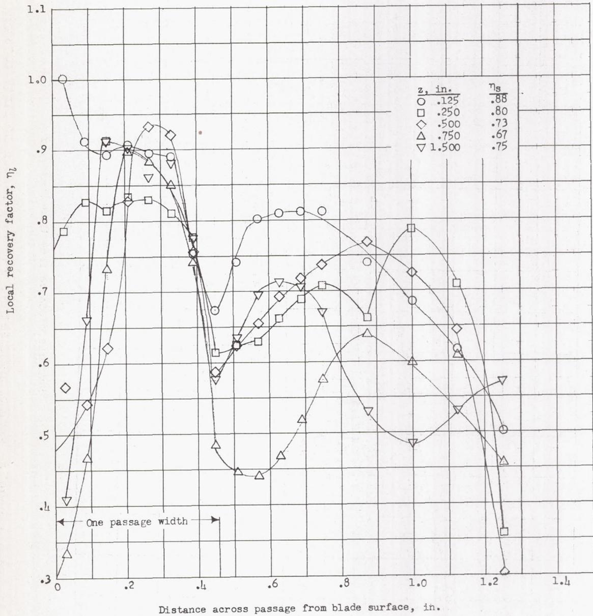
Figure 5.- Local recovery factor for full-contour blades at a floor angle of  $8.4^\circ$ . Both visible passages started.
