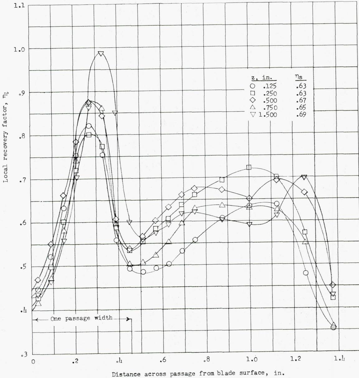
Figure 10.- Local recovery factor for free-streamline blades at a floor angle of  $5.2^\circ$ .
