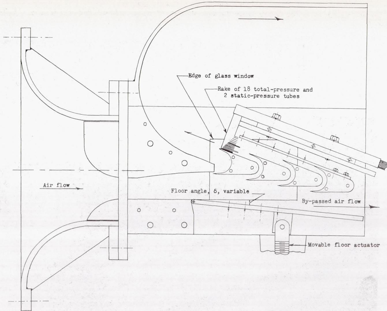
Figure 3.- Sketch of test section with full-contour blade section installed and one wall removed.
