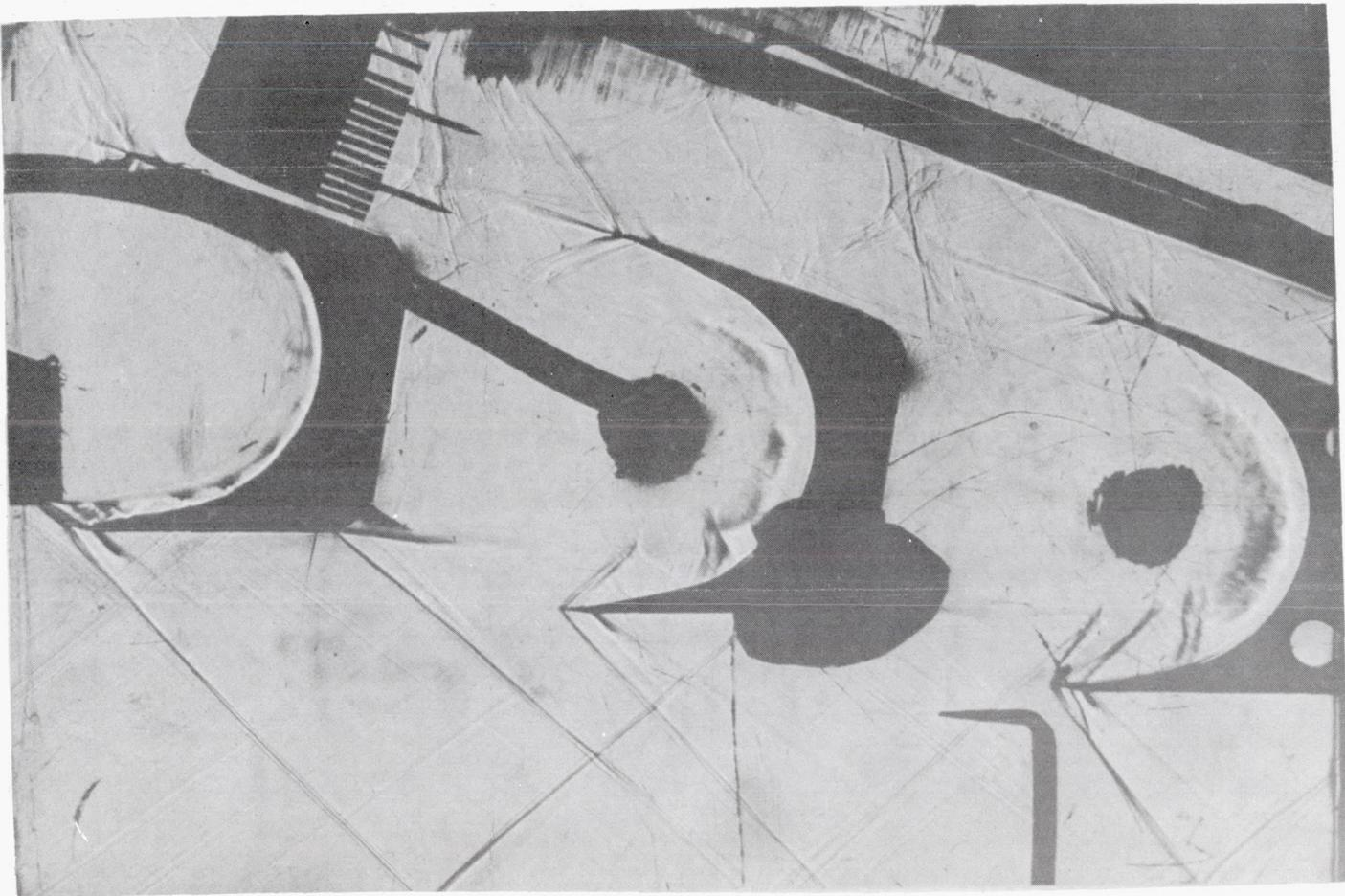
Figure 12.- Schlieren photograph of free-streamline blades at a floor angle of  $2.3^{\circ}$ . Rake is 0.040 inch from tunnel wall. L-57-1619
