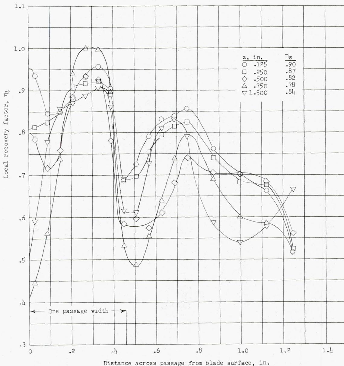
Figure 8.- Local recovery factor for full-contour blades at a floor angle of  $5.2^\circ$ . Only first passage started.
