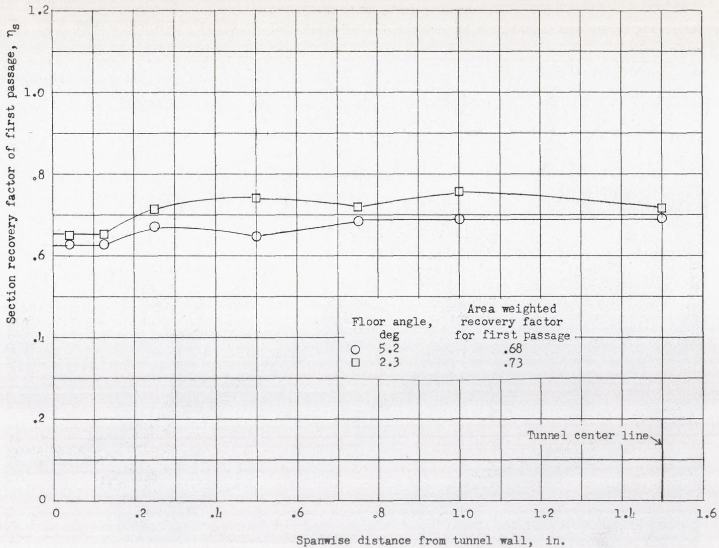
Figure 11.- Spanwise variation of section recovery factor of first passage.
