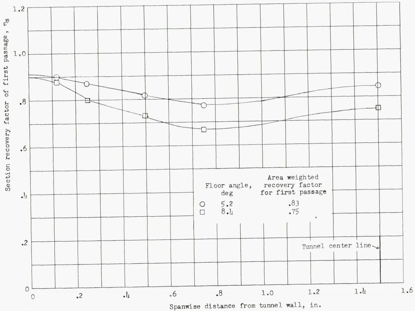
Figure 6.- Spanwise variation of section recovery factor of first passage.
