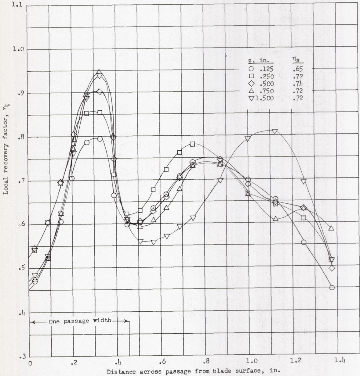
Figure 13.- Local recovery factor for free-streamline blade at a floor angle of  $2.3^\circ$ .
