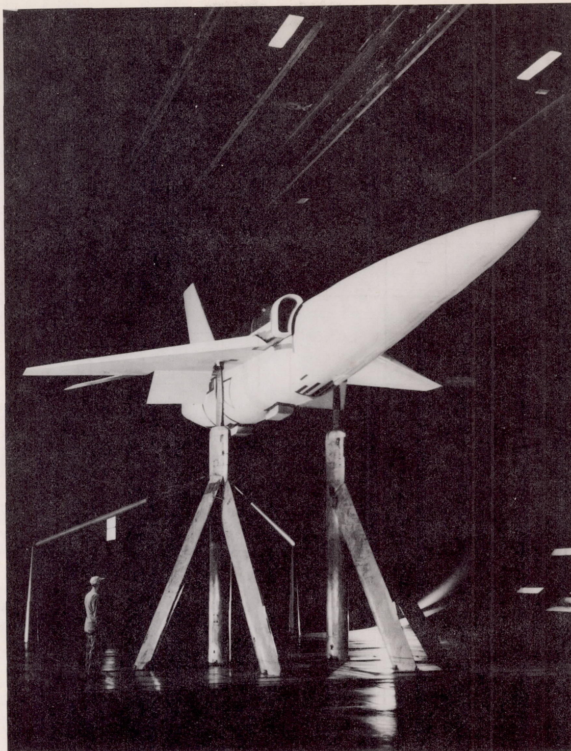
Figure 1.- Photograph of the model mounted in the Ames 40- by 80-foot wind tunnel.
