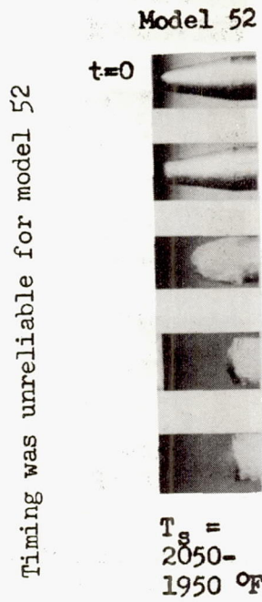
Figure 14.- Behavior of aluminum alloy in hot-air jet.
