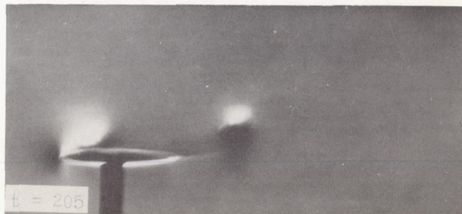
L-57-2785 Figure 4.- Schlieren photographs of configuration 1; \alpha_B = 86^\circ ; jet flow. Time t is given in microseconds.
