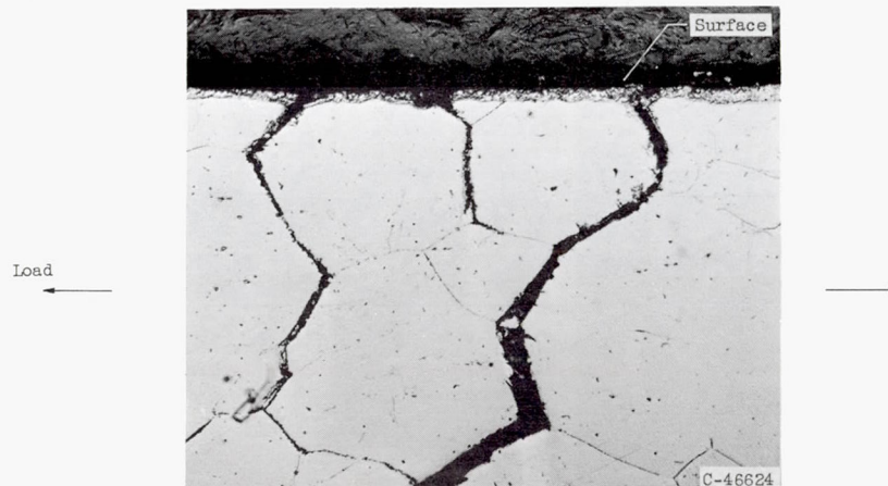
(c) Specimens of group C where coarse grains occur along surfaces.
