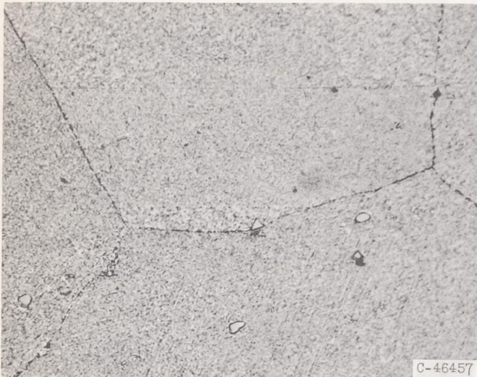
Figure 12. - Typical microstructure of failed buckets. (Lot 3 bucket operated 421 hours.) Original magnification, X750.
