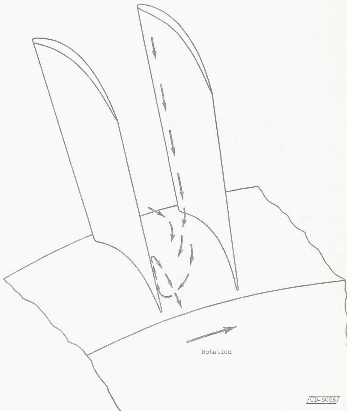
Figure 5. - Flow path of blade losses from pressure-surface boundary layer and contribution to cross-channel flow at hub.
