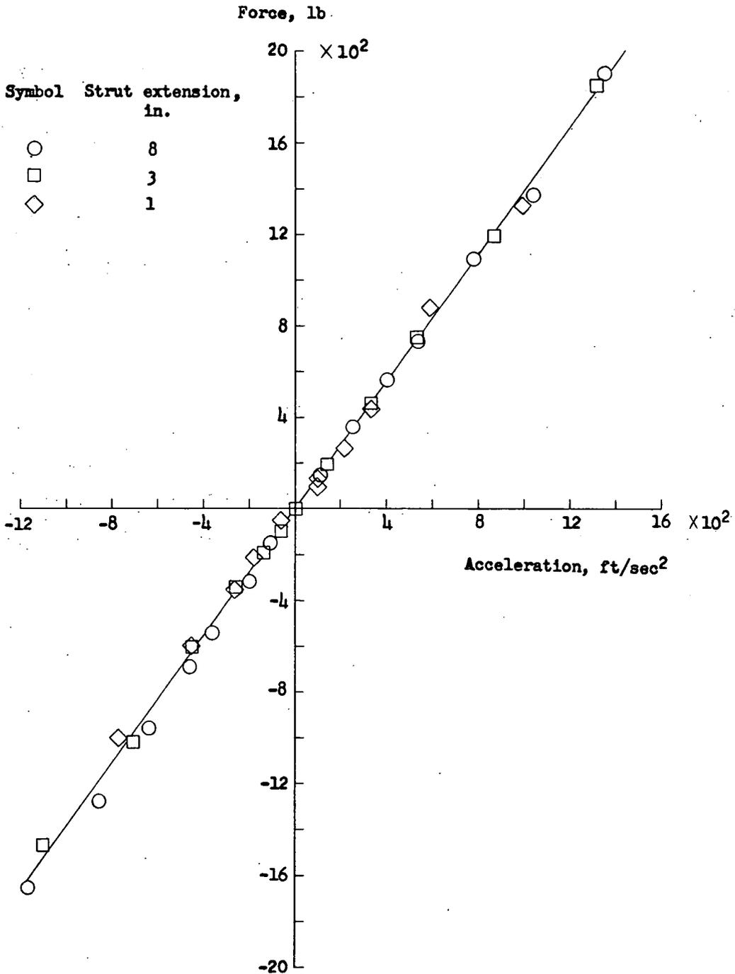
Figure 26.- Variation of horizontal component of force in drag strut with horizontal acceleration of axle during free vibration tests of F-94C nose landing gear.
