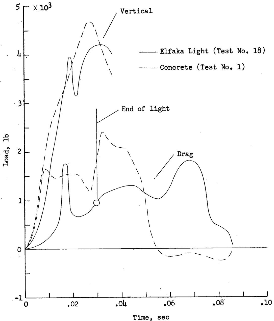
Figure 19.- Comparison of vertical and drag loads developed on F-94C nose gear during landing impacts on concrete and the Elfaka light.
