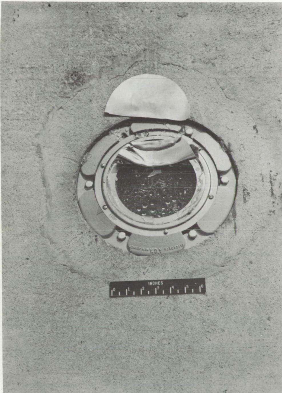
Figure 24.- AGA expendable-top light after F-94C nose wheel roll-over test. L-57-3672
