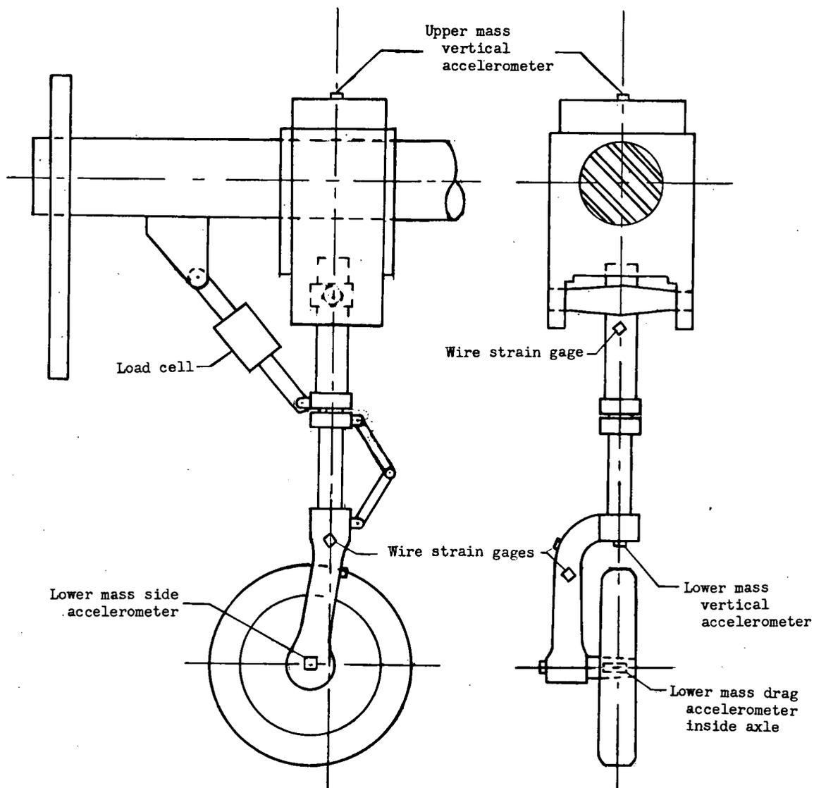
Figure 13.- Sketch of F-94C nose landing gear showing instrument locations.
