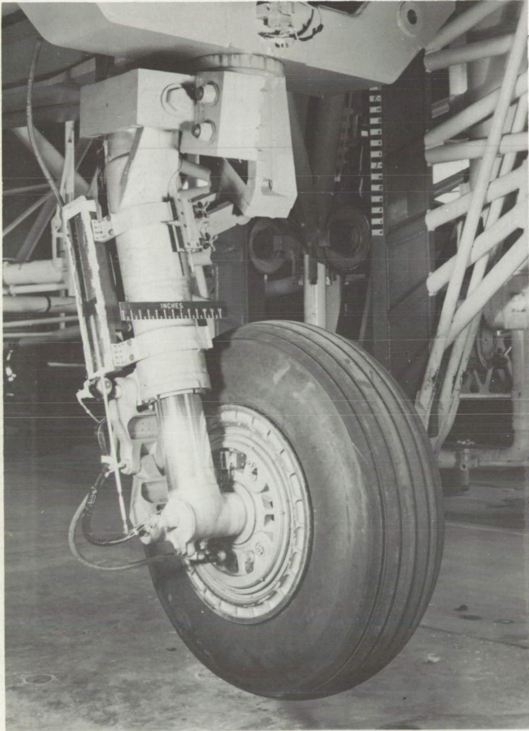
Figure 14.- B-57 main landing gear mounted for test. L-57-1338
