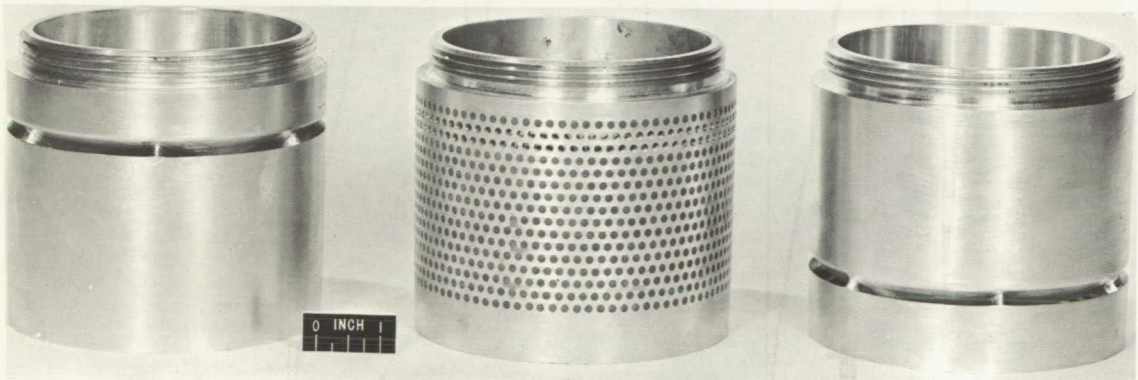
(b) Centerbody constant-area sections showing bleed slots (forward and rear) and perforations.
