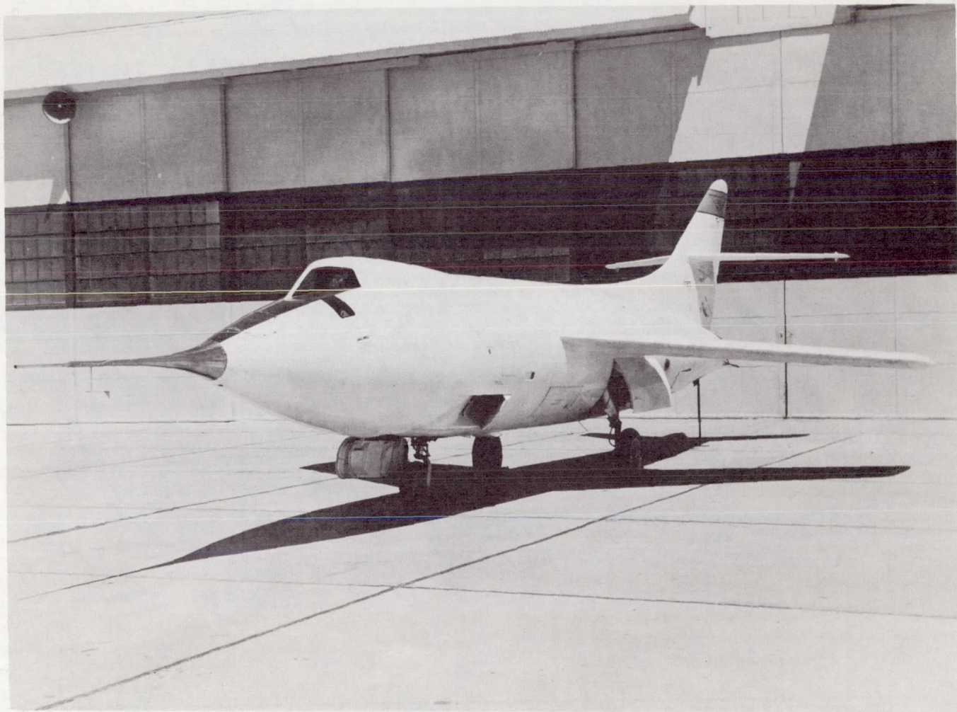
E-488 Figure 1.- Three-quarter front view of Douglas D-558-II airplane. Inboard fences shown installed on wing.
