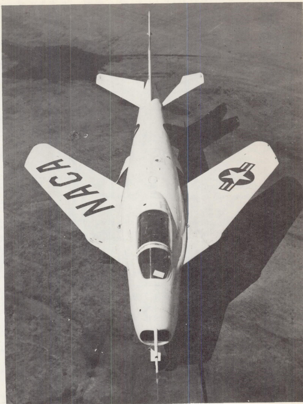
Figure 1.- Photograph of the Bell X-5 research airplane at 58.7^\circ sweepback. E-813
