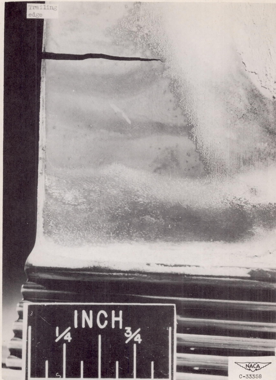
Figure 9. - Rotor blade after spray cooling operation showing trailing edge crack typical of blade failures encountered when large chordwise temperature differences were measured at midspan.
