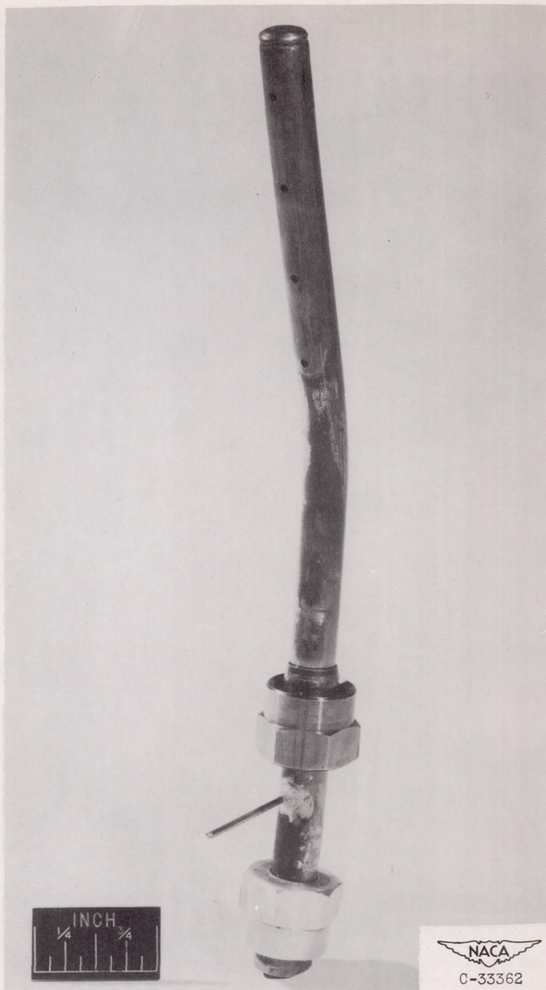
Figure 12. - Inconel spray bar after approximately 1 hour of engine operation at rated speed with and without spray cooling.
