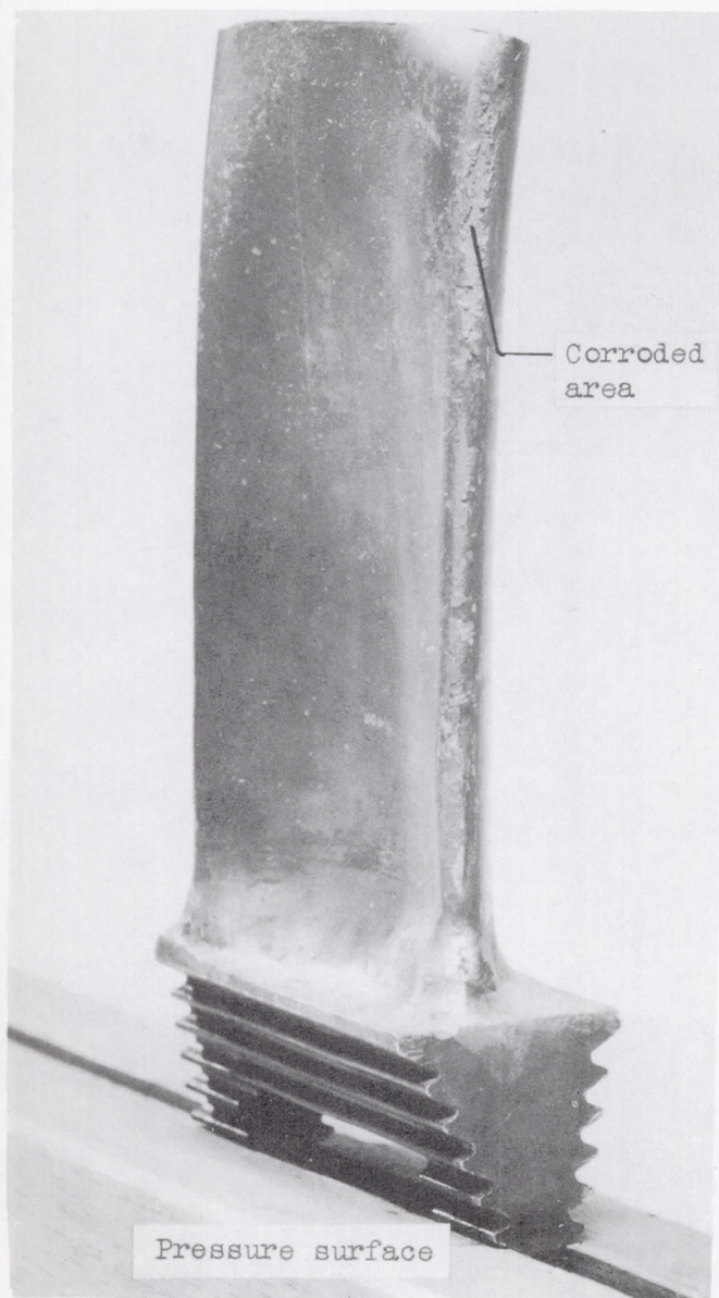
(b) Blade 6 after 44 hours at rated test conditions with coolant-flow ratio of 0.048. Coating chipped and eroded on leading edge and eroded along trailing edge. Leading edge corroded near tip.
