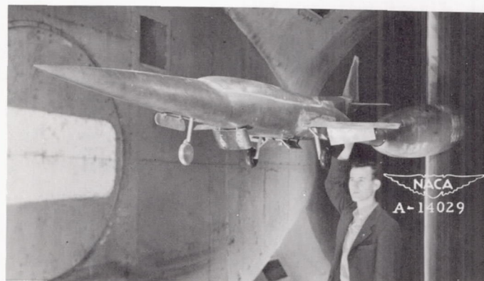
(c) Model with the elongated single airbrake at fuselage station 41.00 inches and with the landing gear extended.
