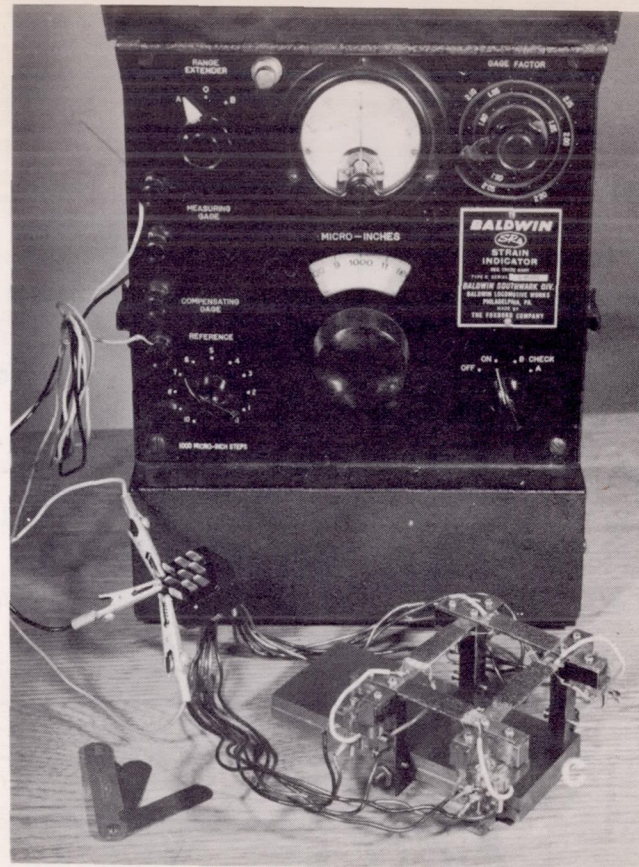
(b) Device for calibrating clip gage.
