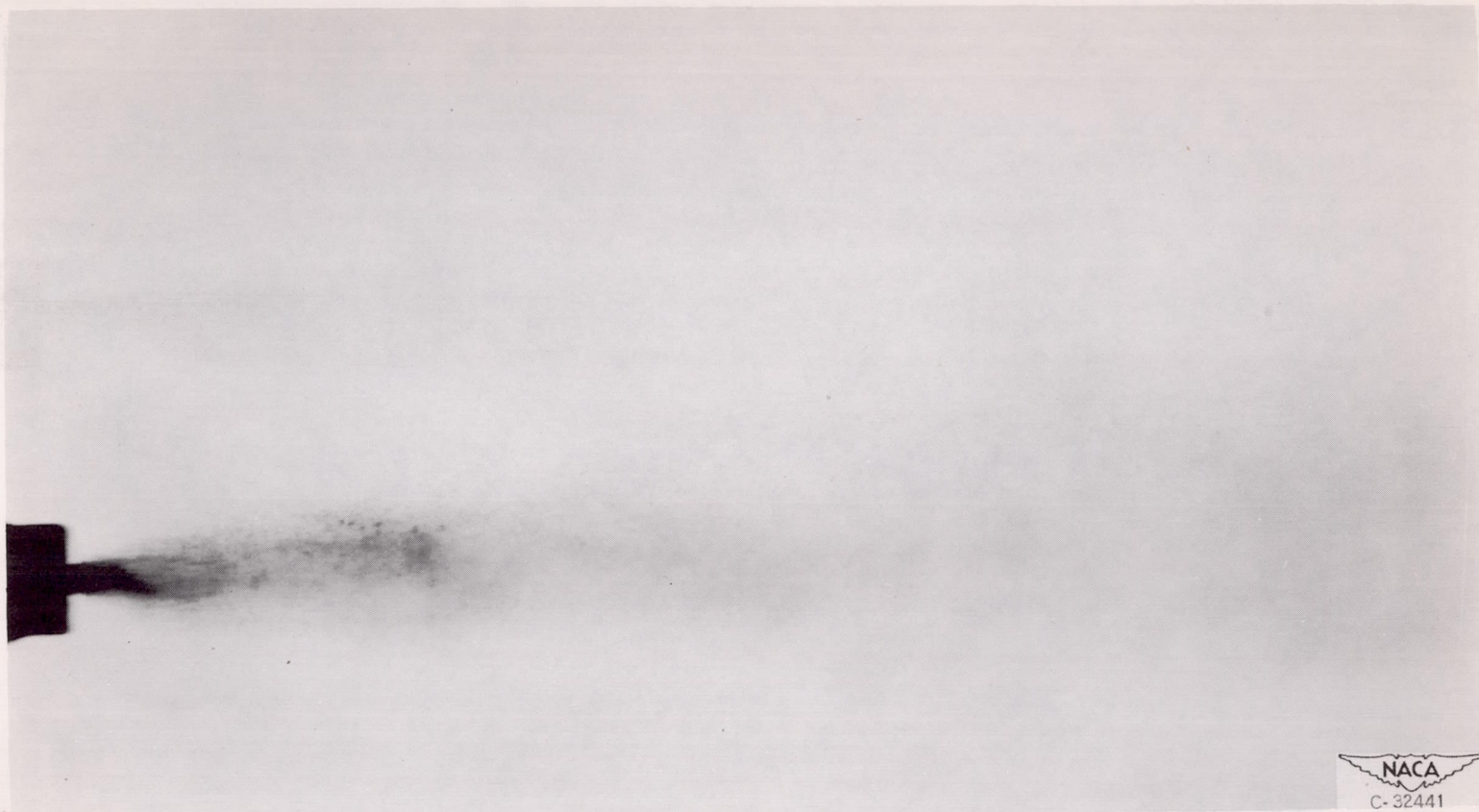
(b) Fuel V, fuel oil 4 plus 50 percent by weight 13-micron magnesium; viscosity, 75 centipoises at 30° C.
