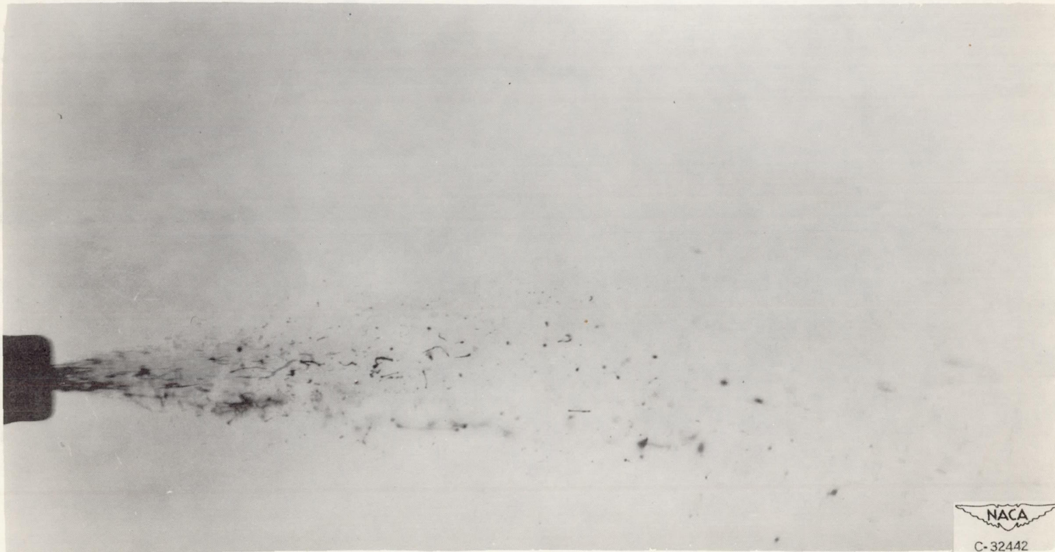
(c) Fuel XII, 50 percent by weight 13-micron magnesium in MIL-F-5624A grade JP-4 fuel plus 0.4 percent-gel; viscosity, 22,750 centipoises at 30° C.
