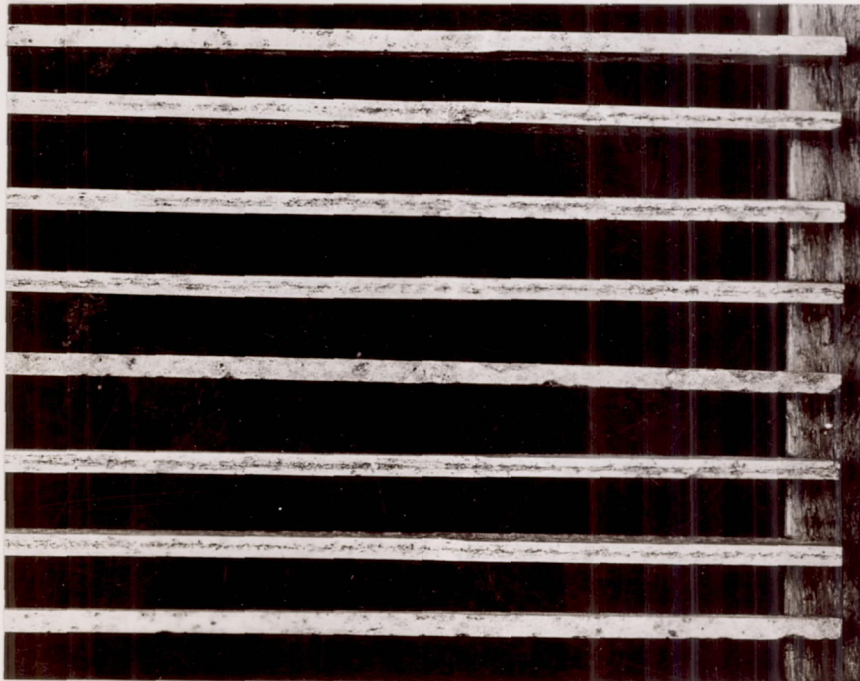
Fig.1 Severe intercrystalline corrosion magnified to 100X.
