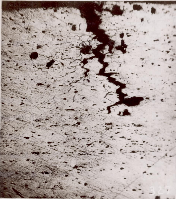
Fig.1 Severe intercrystalline corrosion magnified to 100X.
