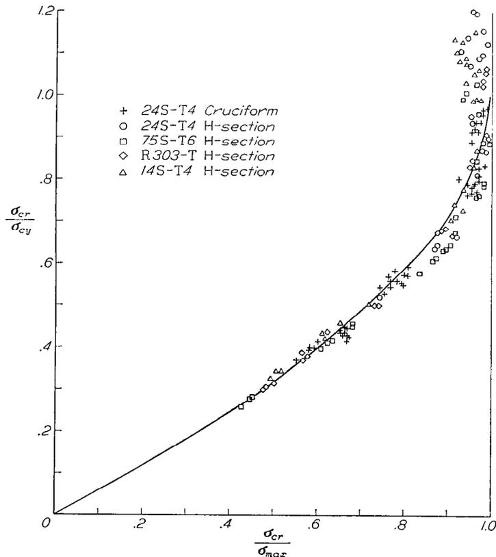
FIGURE 7.—Comparison of theoretical curve for the maximum strength of 24S-T4 aluminum alloy cruciforms with test results. Compressive yield stress  $\sigma_{cy}$  = 46 ksi. (Experimental values for H-sections of various aluminum alloys have been added for comparison with the theoretical curve.)
