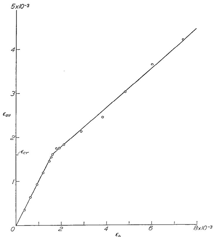
FIGURE 5.—Theoretical middle-surface strain relation between  $\epsilon_{av}$ ,  $\epsilon_h$ , and  $\epsilon_{cr}$  for a hinged flange compared with experiment. ( $\epsilon_{av} = \frac{4}{9}\epsilon_h + \frac{5}{9}\epsilon_{cr}$  for  $\epsilon_{av} > \epsilon_{cr}$ .)
