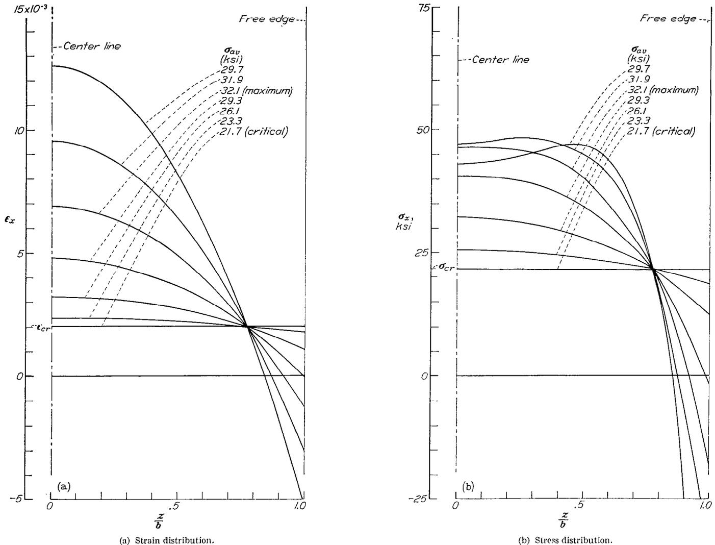
FIGURE 8.—Theoretical middle-surface strain and stress distribution across a flange at the quarter-length station along a typical cruciform.  $\frac{b}{t} = 14$ ;  $\frac{L}{b} = 12$ .
